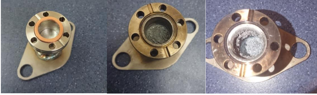
Figure 13. Illustration of the propellant tank before the tests, after the initial tests, and at the end of the testing.
