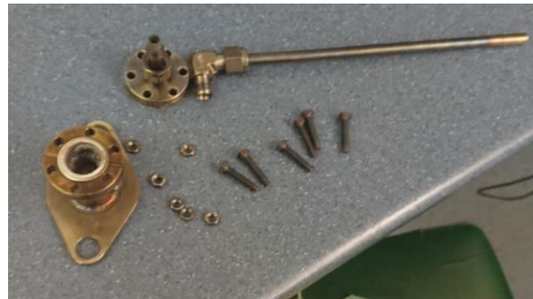
Figure 8. The manufactured propellant tank, top flange of propellant tank, and simple feedline.
