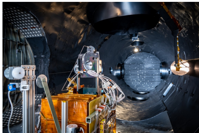
Figure 8. Recently reactivated Vacuum Facility 11 vacuum chamber with thrust stand installed.
