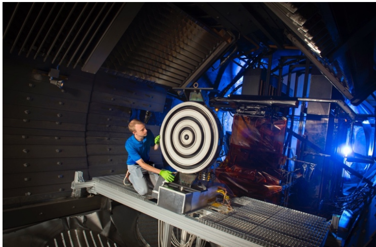
Figure 6. XR-100 installed in NASA Glenn Research Center Vacuum Facility 5 vacuum chamber.
