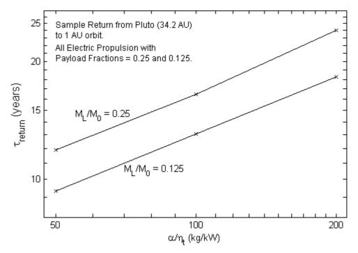
Figure 4. Sample return time from Pluto (departure in 2020) to a 1 AU Earth orbit as a function of EP powerplant specific mass for different payload mass fractions ( $M_L/M_O$ ) of the return rocket.
