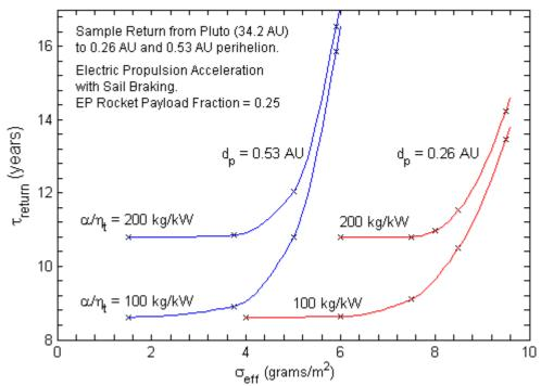
**Figure 5.** Sample return time from Pluto (departure in 2020) with sail deceleration to 0.26 AU and 0.53 AU perihelion points versus sailcraft loading. Results for different powerplant specific masses of the EP return rocket are illustrated.
