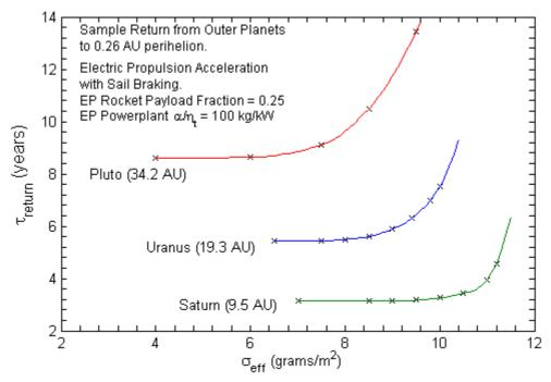
**Figure 6.** Sample return time from the outer planets with sail deceleration to 0.26 AU perihelion point versus sailcraft loading. The powerplant specific mass of the EP return rocket is 100 kg/kW in these examples.
