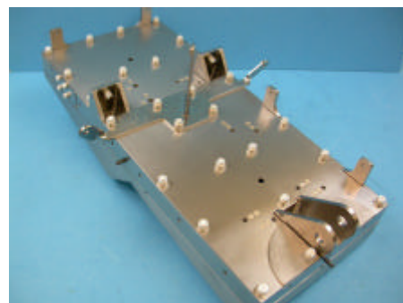
Figure 4. Mobile platform box structure (bottom view)
