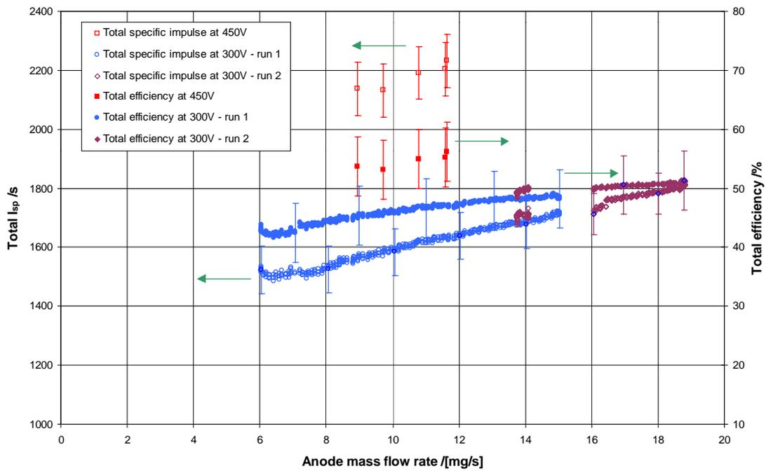
**Figure 10 – Total specific impulse and total efficiency vs. anode mass flow rate**
