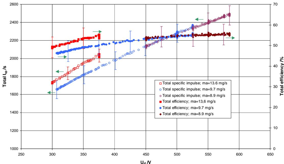
**Figure 11 – Total specific impulse and total efficiency vs. discharge voltage**
