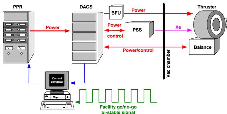
*Figure 5 - Electrical Power and Data Acquisition Architecture*
