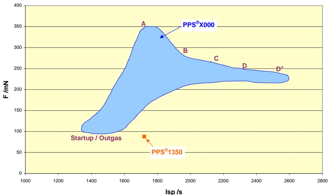
**Figure 8** – Thrust vs.  $I_{sp}$  in reference configuration
