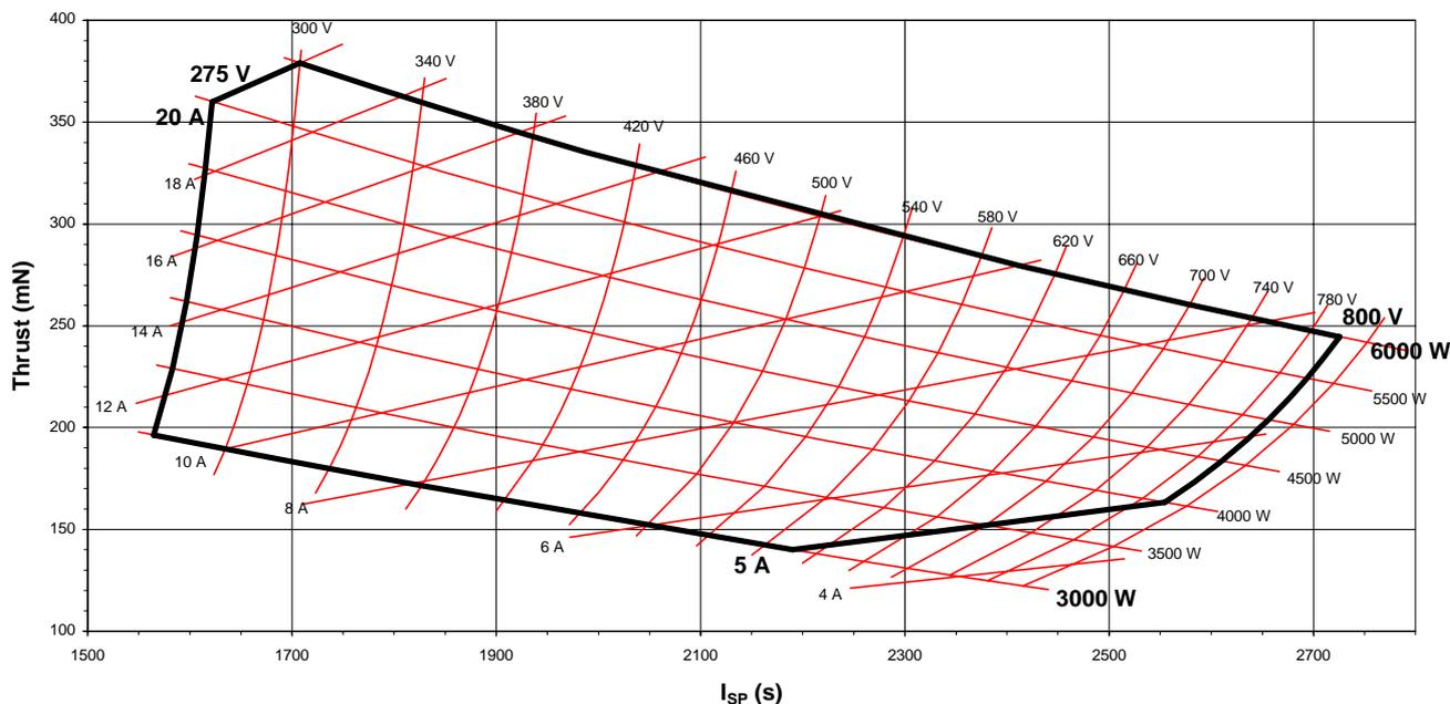
**Figure 2 - PPS<sup>®</sup> X000 design operating range.**
