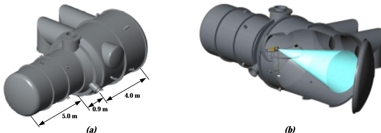
***Figure 3 - LEEP2 vacuum test facility chamber at QinetiQ.***
