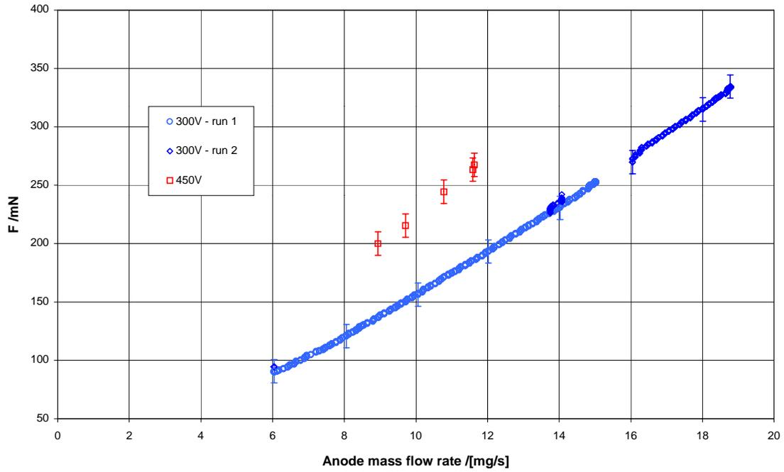
**Figure 9 – Thrust vs. anode mass flow rate**
