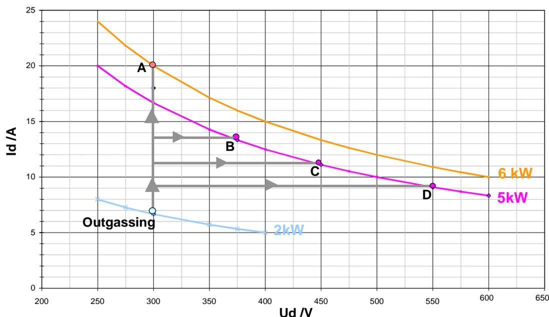
**Figure 6 – PPS<sup>®</sup>X000 outgassing and characterisation points**
