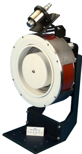
Figure 1 – Photograph of the NASA-173Mv2 Hall effect thruster.
