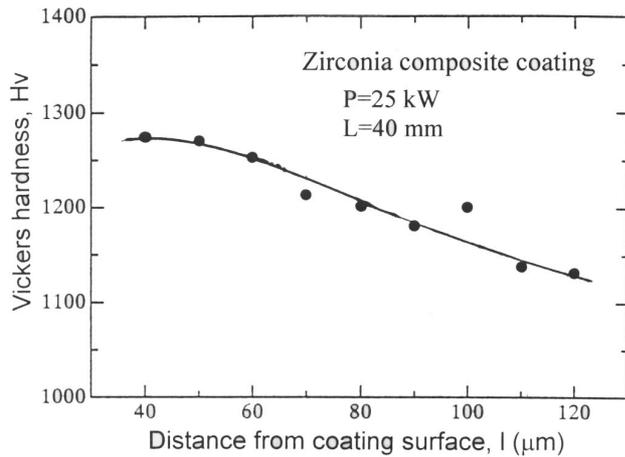
**Fig.6** Distributions of Vickers hardness on cross section of zirconia composite coatings sprayed by 30 times traverse at  $L=40\text{mm}$  when  $P=25$  kW.
