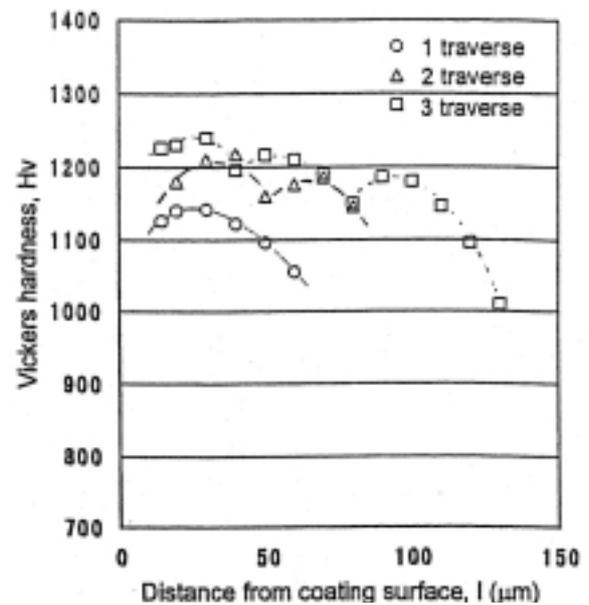
Fig.2 Distributions of Vickers hardness on cross section of zirconia composite coatings sprayed at  $L=40$ mm when  $P=25$  kW. Data plots: 1 time, 2 times and 3 times traverse.
