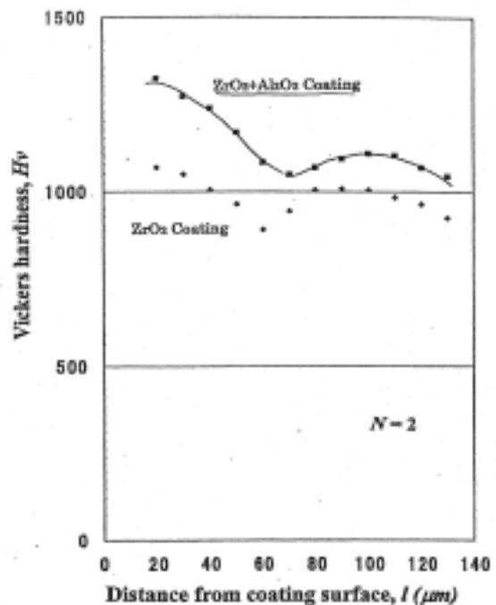
**Fig.5** Distributions of Vickers hardness on cross section of zirconia composite coatings sprayed by 2 times traverse at  $L=40$ mm when  $P=25$  kW.
