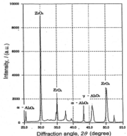
**Fig.8** X-ray diffraction patterns of zirconia composite coating for 2-times traverse in Fig.6.
