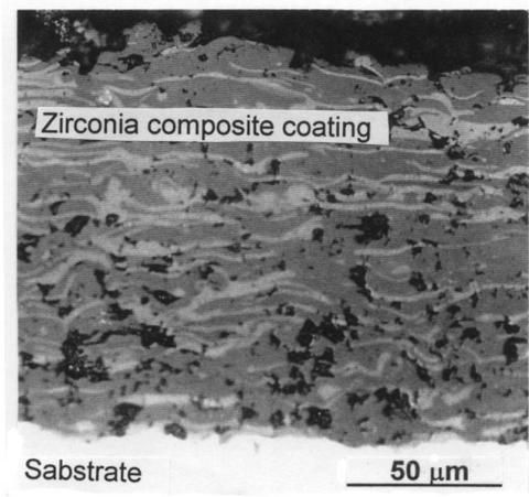
**Fig.7** Microphotograph of the cross section of  $\text{ZrO}_2$  composite coatings sprayed by 33 times traverse at  $L=40\text{mm}$  when  $P=25$  kW.
