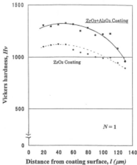
**Fig.4** Distributions of Vickers hardness on cross section of zirconia composite coatings sprayed by 1 time traverse at  $L=40$ mm when  $P=20$  kW.
