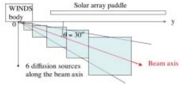
Figure 4: Schematic picture of diffusion source along the thruster plume.
