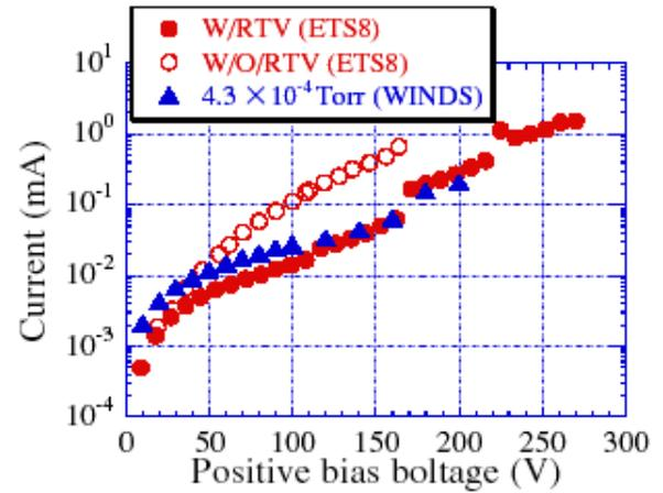
Figure 13: Electron current collected at different bias voltages.
