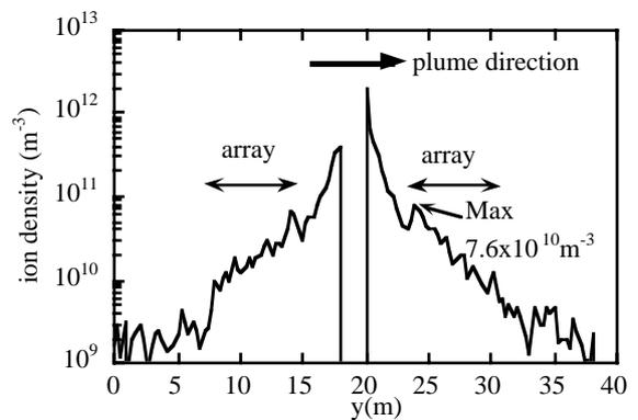
Figure 9: Distribution of ion density along  $y$  axis crossing the thruster exit on  $xy$  plane shown in Fig. 8w
