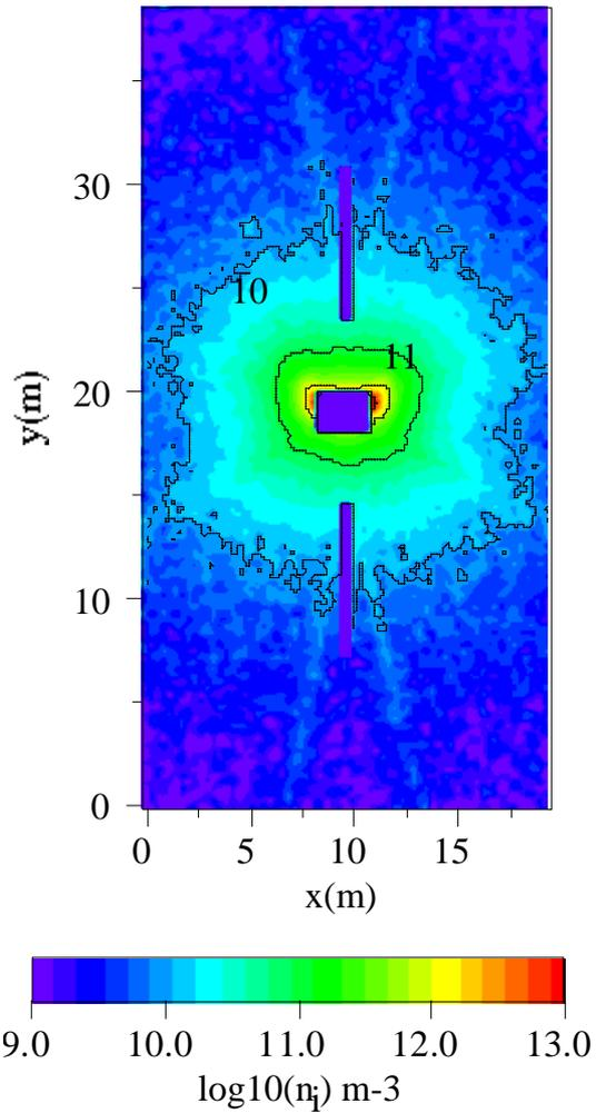
Figure 8: Distribution of ion density on  $xy$  plane when the solar array paddle faces the  $x$  axis.
