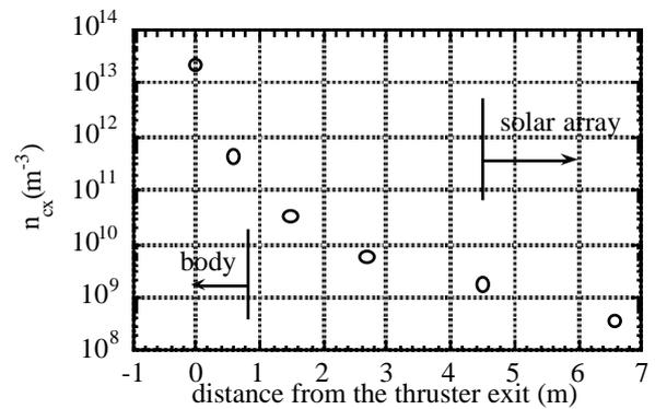
Figure 5: Density of CEX ions at each diffusion source along the thruster plume. The distance is along  $y$  axis shown in Fig. 4
