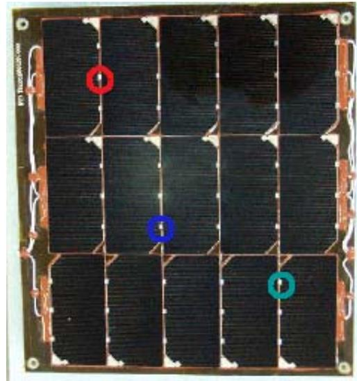
Figure 12: Photograph of solar array coupon used in the laboratory experiment.
