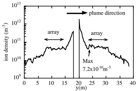
Figure 11: Distribution of ion density along  $y$  axis crossing the thruster exit on  $xy$  plane shown in Fig. 10
