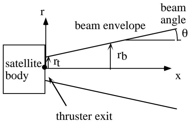
Figure 2: Coordinate system used to calculate the distribution of beam ion and neutral density inside the thruster plume.
