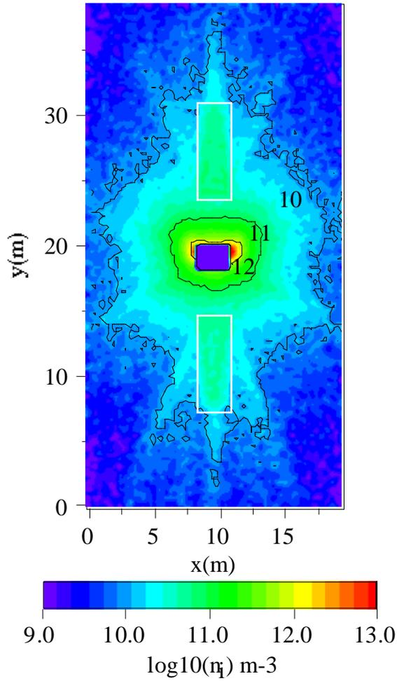
Figure 10: Distribution of ion density on  $xy$  plane when the solar array paddle faces the  $z$  axis.
