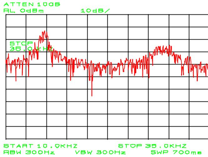
**Fig. 12:** Low frequency spectrum for thruster operation at DC mode (Discharge voltage= 230V)
