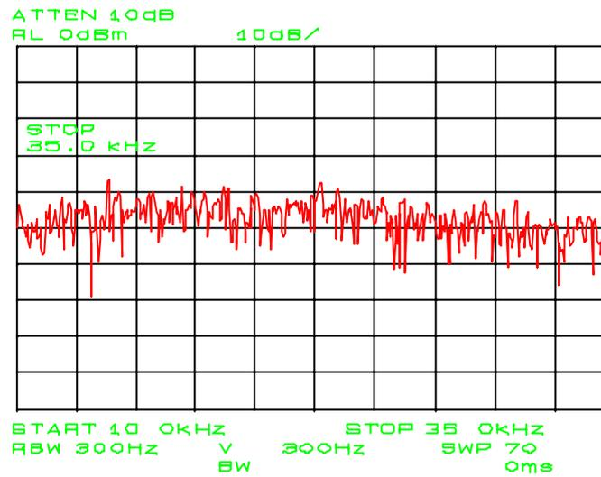
**Fig. 13:** Low frequency spectrum for thruster operation at **100W** (Discharge voltage= 230V)
