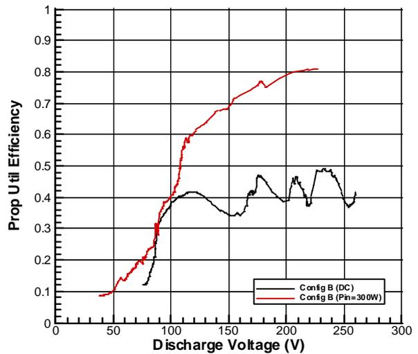
**Fig. 7:** Propellant Utilization Efficiency
