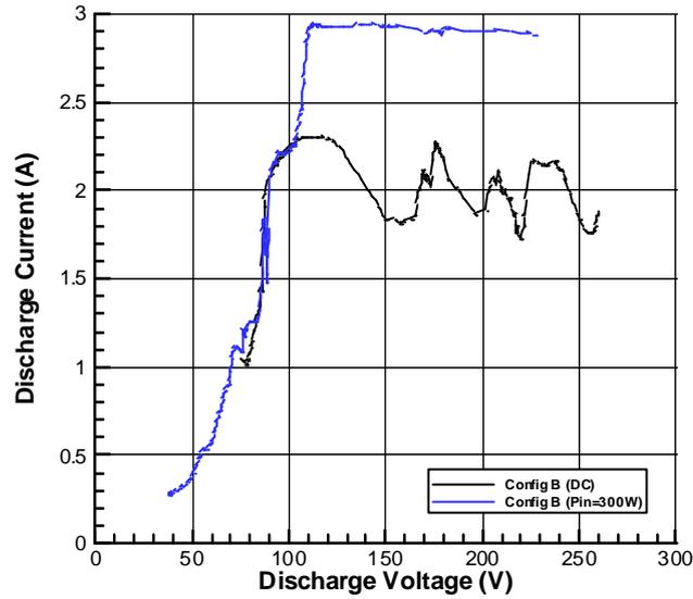
**Fig. 5:** VI curve for DC and microwave mode cases
