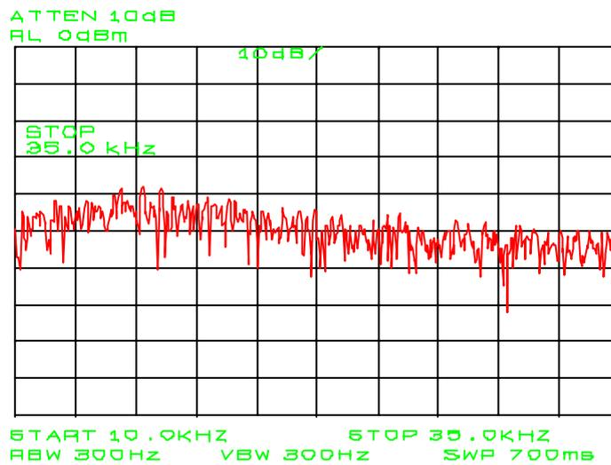
**Fig. 14:** Low frequency spectrum for thruster operation at **300W** (Discharge voltage= 230V)
