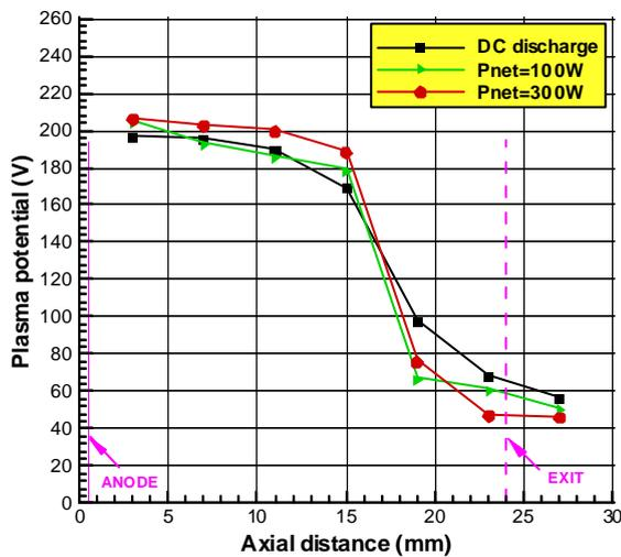
**Fig. 8:** Plasma potential variation along channel (DC mode, 100W & 300W  $\mu$ wave input mode)
