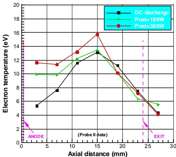
**Fig. 10:** Electron temperature variation (DC, 100W $\mu$  & 300W $\mu$ )
