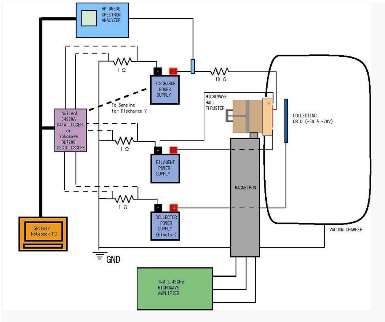
**Fig. 15:** Overall experimental system
