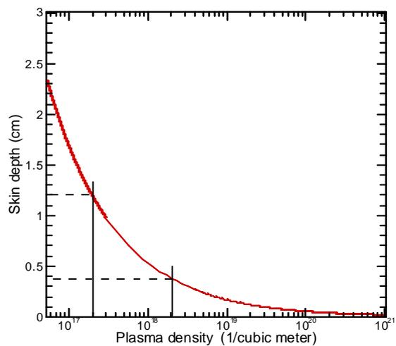
**Fig. 11:** Microwave penetration dependency on plasma density (Xe).
