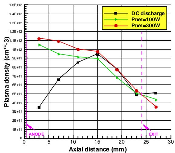
**Fig. 9:** Plasma density variation (DC, 100W $\mu$  & 300W $\mu$ )
