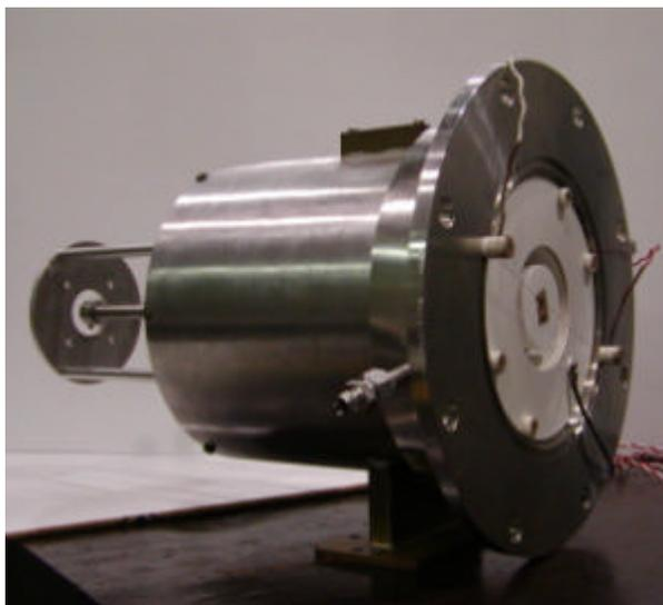
**Fig. 1:** Microwave Hall thruster: Prototype II
