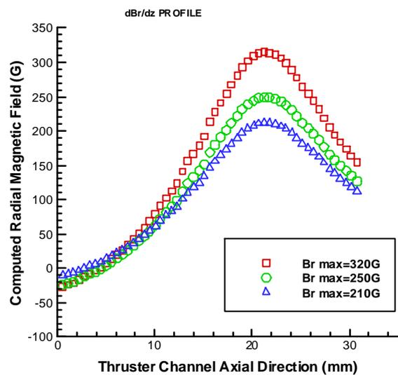
**Fig. 2:** Calculated radial magnetic field along the central axis of accelerating channel.
