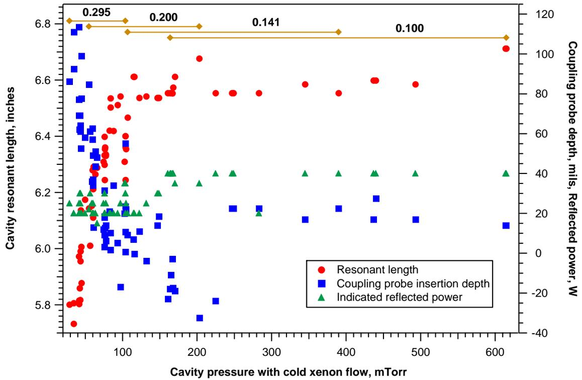
Figure 6. Effect of decreasing pressure on cavity tuning.
