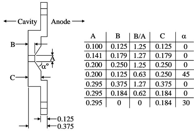
Figure 5. Section view of aperture plate (dimensions in inches).
