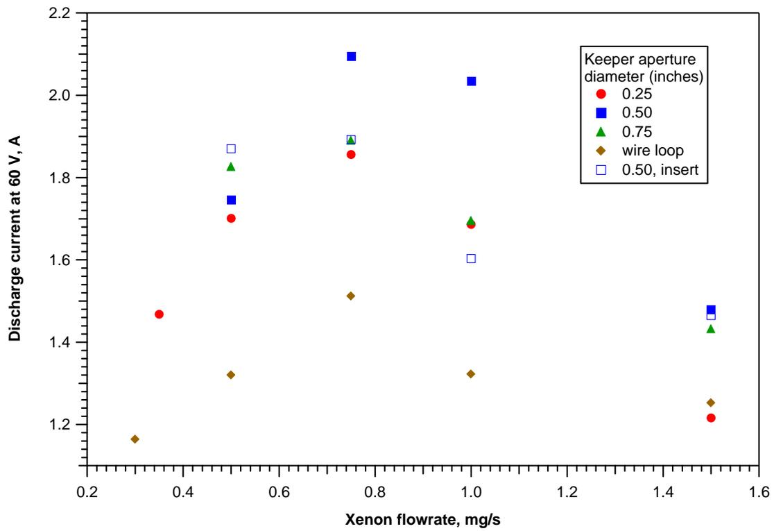
Figure 9. Effect of enclosed keeper on anode current at 60 V with 0.295 inch diameter extraction aperture.
