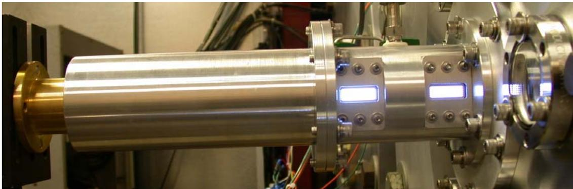
Figure 2. Cavity with xenon plasma.
