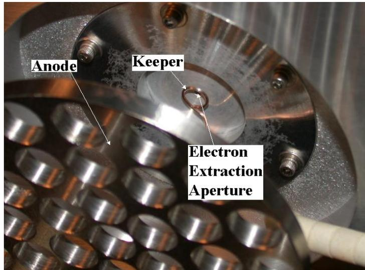
Figure 3. Anode and wire loop keeper.
