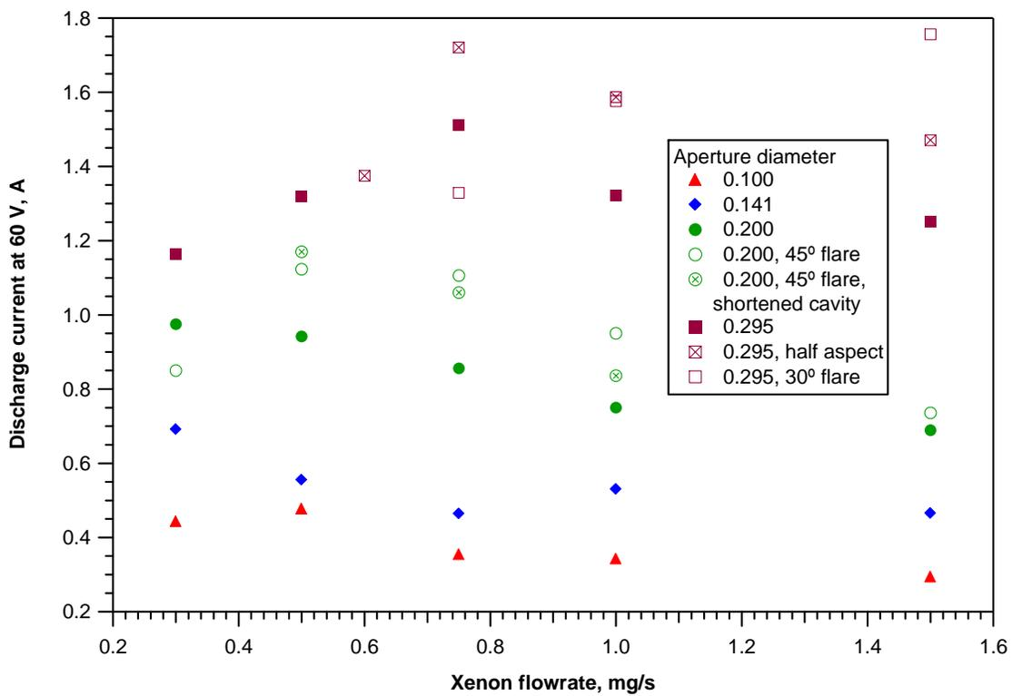
Figure 4. Effect of aperture geometry on anode current at 60 V.
