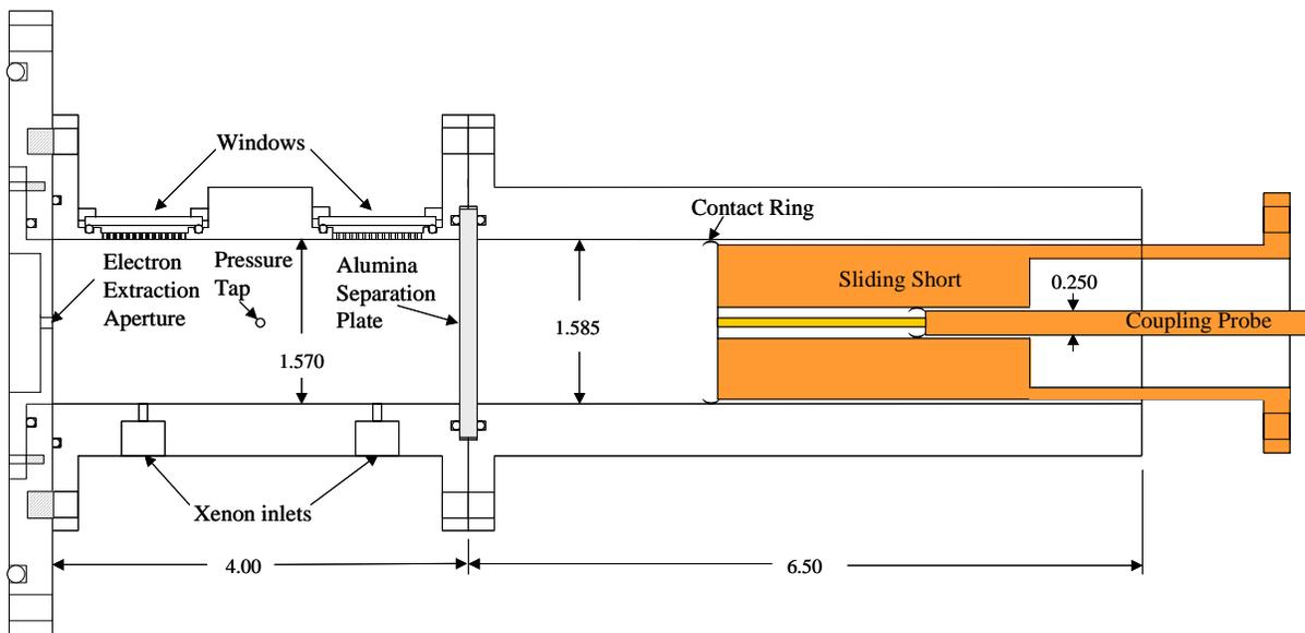
Figure 1. Section view of resonant cavity (dimensions in inches).
