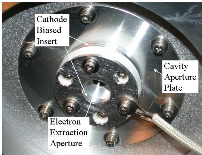
Figure 13. Enclosed keeper with cathode biased insert.
