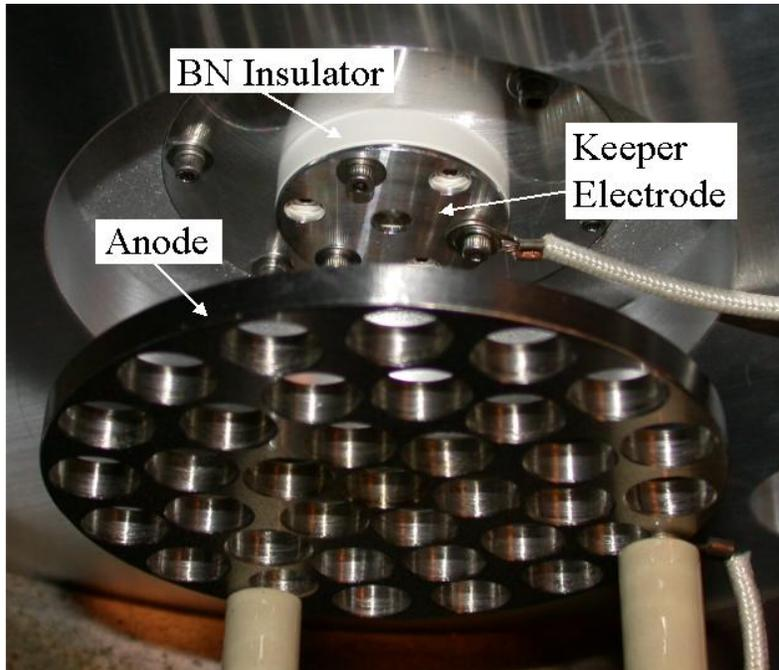
Figure 8. Enclosed keeper.
