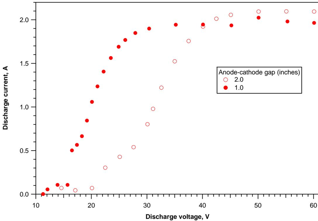
Figure 11. Effect of anode-cathode gap, 0.295 aperture with 0.50 enclosed keeper, 0.75 mg/s, keeper off.
