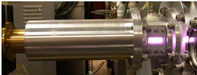
Figure 7. Shortened cavity with air plasma.
