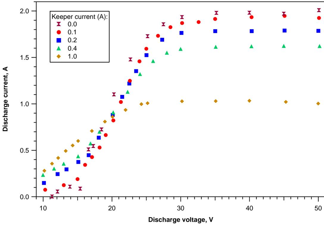
Figure 10. Effect of keeper current, 0.295 aperture with 0.50 enclosed keeper, 0.75 mg/s.
