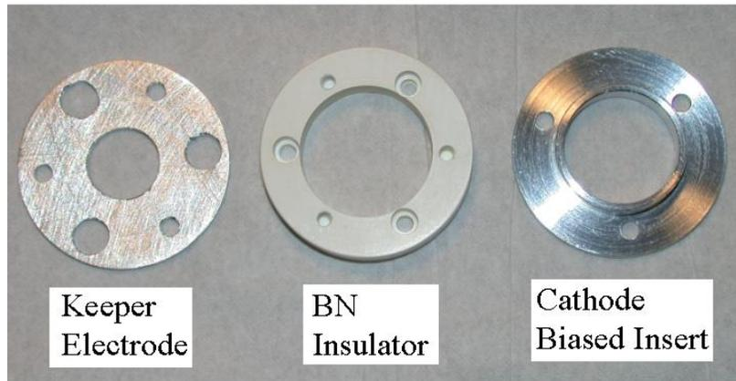
Figure 12. Parts for enclosed keeper with cathode biased insert.
