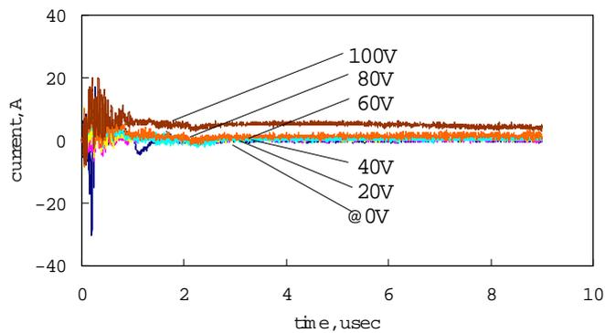
Fig.5 Temporal variations of discharge current of a coaxial thruster for low voltage conditions.
