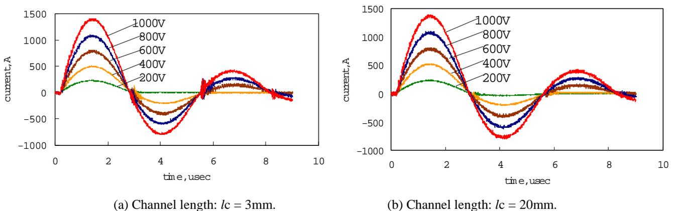
Fig.6 Temporal variations of discharge current of rectangular thrusters for high voltage conditions.
