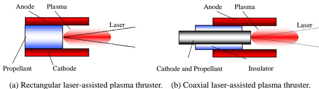
Fig.1 Schematics of laser-assisted plasma thrusters.
