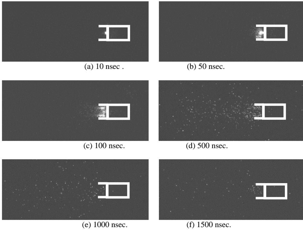
Fig.8 ICCD images (gate width: 10nsec) of exhaust plasma plume from a rectangular thruster (channel length: 3 mm, anode: upper plate) for charged voltage: 0 V.
