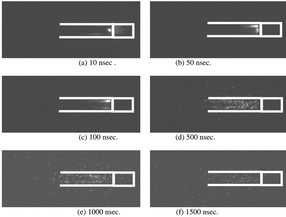
Fig.10 ICCD images (gate width: 10nsec) of exhaust plasma plume from a rectangular thruster (channel length: 20 mm, anode: upper plate) for charged voltage: 0 V.
