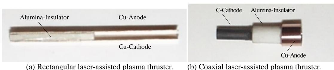
Fig.2 Photos of laser-assisted plasma thrusters.
