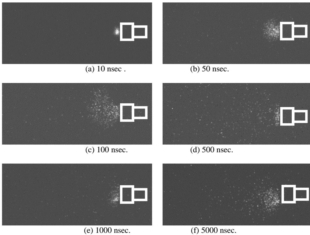
Fig.13 ICCD images (gate width: 10nsec) of exhaust plasma plume from a coaxial thruster (channel length: 2 mm) for charged voltage: 1000 V.
