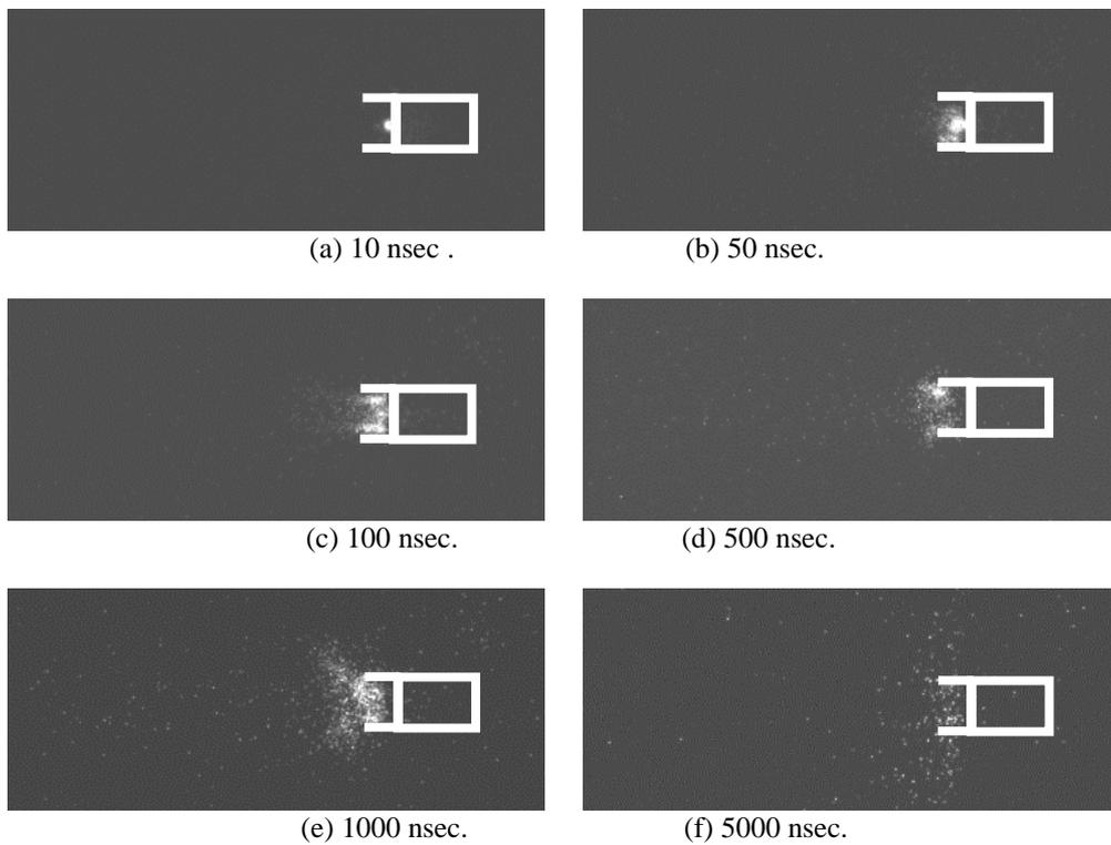
Fig.9 ICCD images (gate width: 10nsec) of exhaust plasma plume from a rectangular thruster (channel length: 3 mm, anode: upper plate) for charged voltage: 1000 V.
