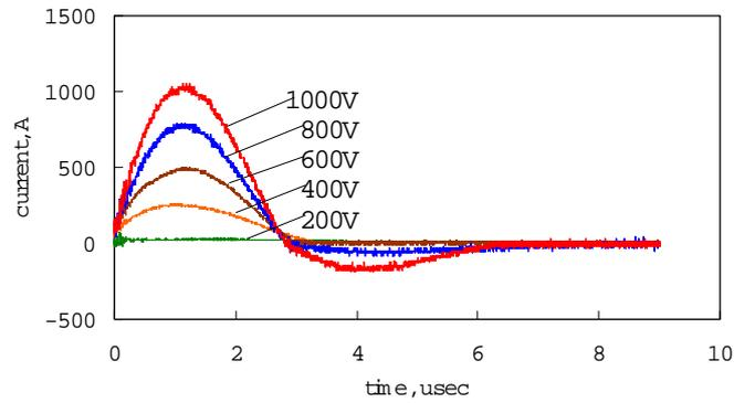
Fig.7 Temporal variations of discharge current of a coaxial thruster for high voltage conditions.
