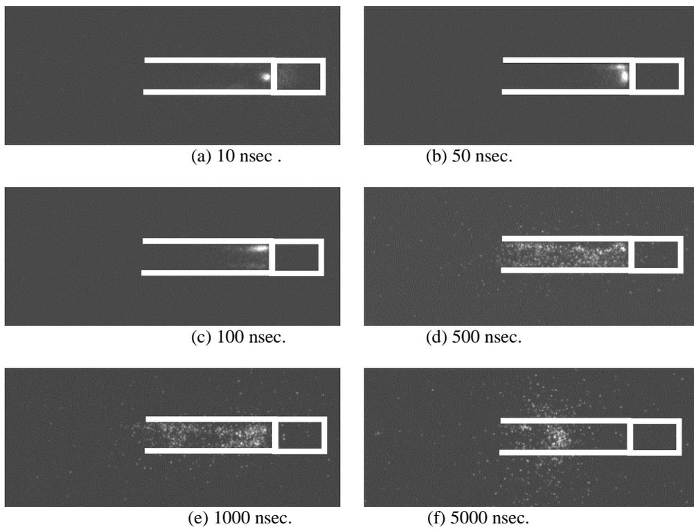
Fig.11 ICCD images (gate width: 10nsec) of exhaust plasma plume from a rectangular thruster (channel length: 20 mm, anode: upper plate) for charged voltage: 1000 V.
