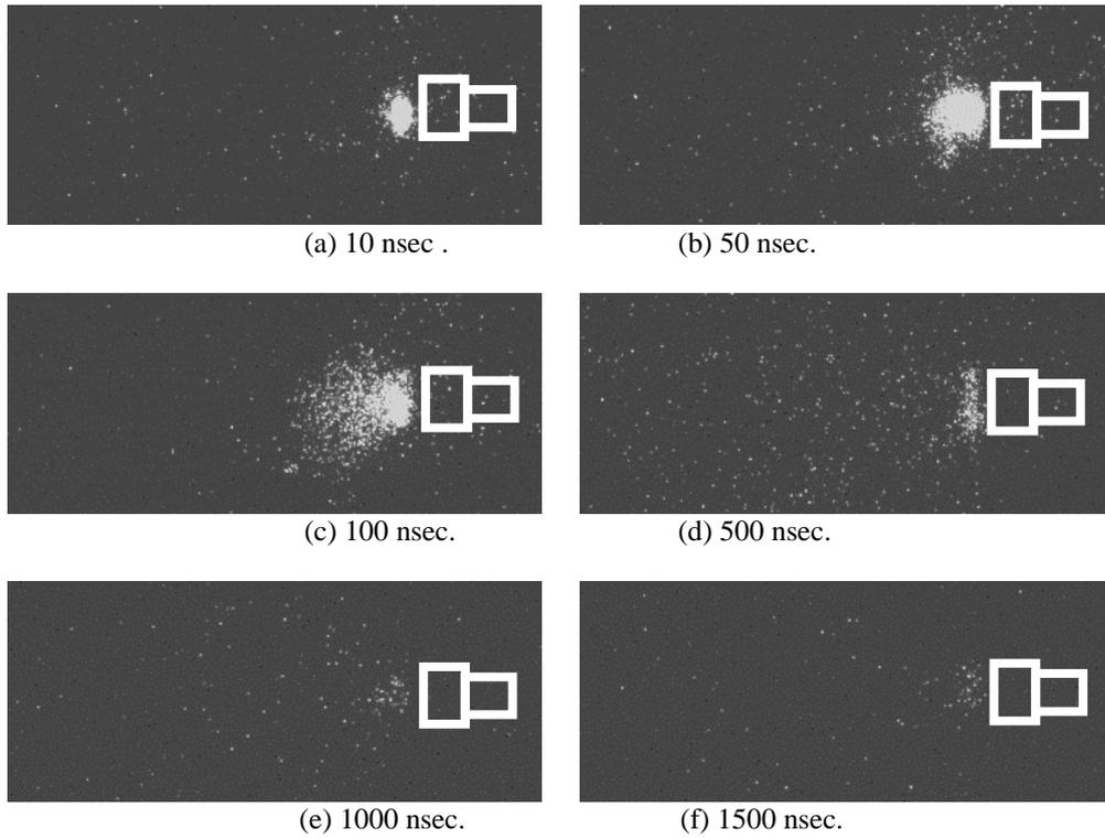
Fig.12 ICCD images (gate width: 10nsec) of exhaust plasma plume from a coaxial thruster (channel length: 2 mm) for charged voltage: 0 V.
