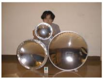
Fig. 2 EMCs of 220 mm, 430 mm, and 640 mm in diameter
