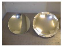
Fig. 1 Mold (left) and Ultra-light EMC (right)
