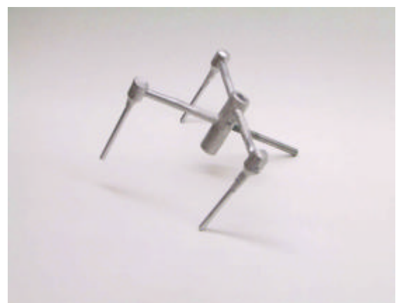
Fig. 7 Mini-Thruster Made of SC-Mo with Outer Dia of 5 mm and Cavity Dia. of 3 mm
