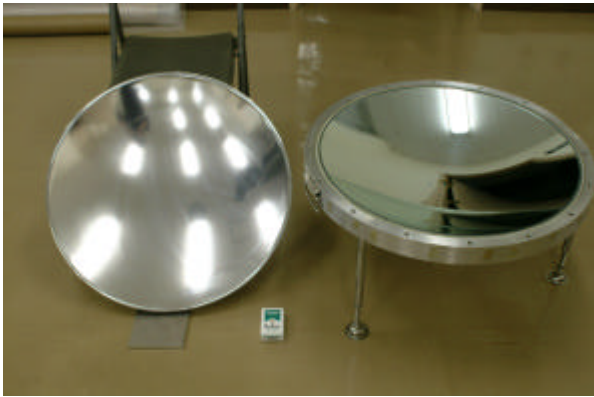
Fig. 12 Glass Mirror as the Mold (640 mm in Dia. and 250 mm in Focal Length) and Film Mirror
