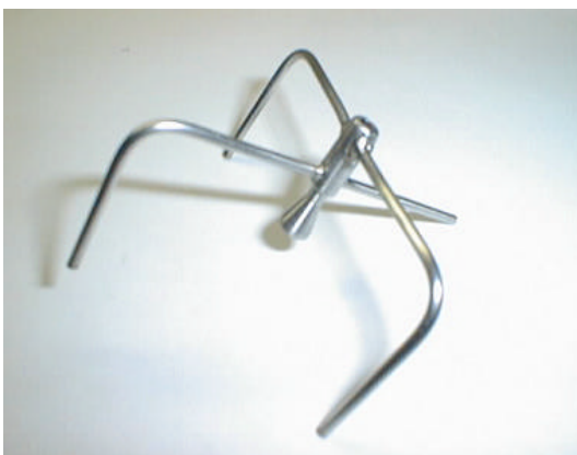
Fig. 6 Mini-Thruster Made of Stainless Steel SUS 316 with Outer Dia. of 5 mm and Dia. of 4 mm
