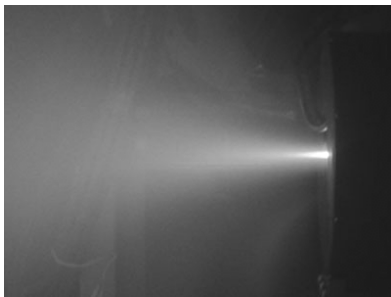
(a) Specific impulse: 450 sec Discharge current: 25A Applied field: 0.15T Mass flow rate: 3mg/s (Ar) Anode: 4
