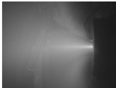
(b) Specific impulse: 300 sec Discharge current: 25A Applied field: 0.15T Mass flow rate: 5mg/s (Ar) Anode: 4
