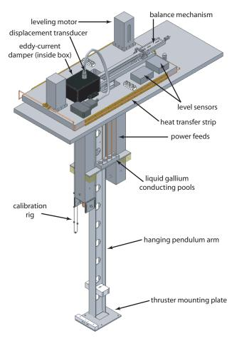
Figure 2. Schematic illustration of the VAHPER thrust stand components.
