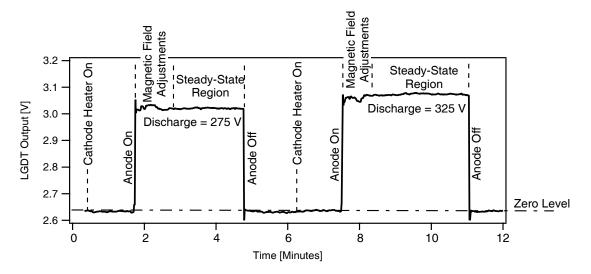
Figure 4. Raw LGDT output data as a function of elapsed time for two thruster operating points.
