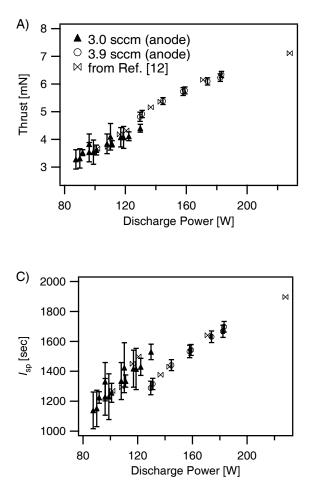
Figure 5. Performance measurements for a 3 cm cylindrical Hall thruster: A) Thrust, B) Anode Efficiency, C)  $I_{\rm sp}$  as a function of discharge power. The error bars represent a 95% (2 $\sigma$ ) confidence interval. No error bars are displayed on the data from Ref. [12].
