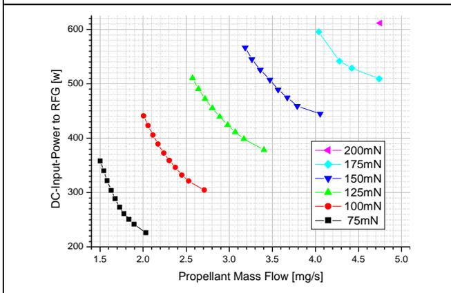
**Fig. 4 (Left)** Operational bandwidth: The Thruster is fully operable at any thrust level over a wide range of propellant mass flow. (Data of laboratory engine to demonstrate engine behavior, not representing the performance of flight type)
