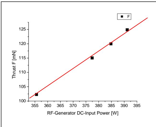
**Fig. 3** Linearity between thrust and RF-power
