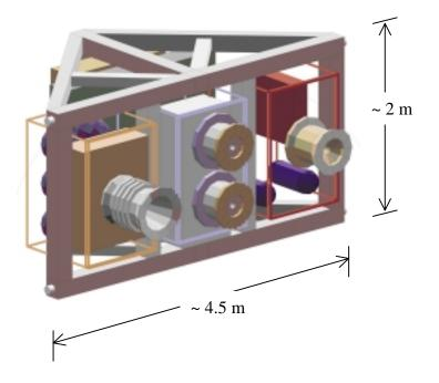
Figure 1: Concept for an International Space Station Electric Propulsion Test Facility
