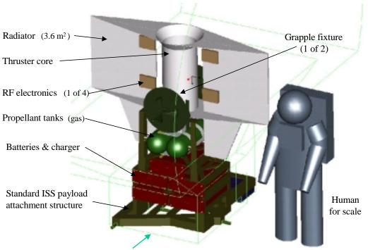
Designed to fit standard ISS external payload envelope
