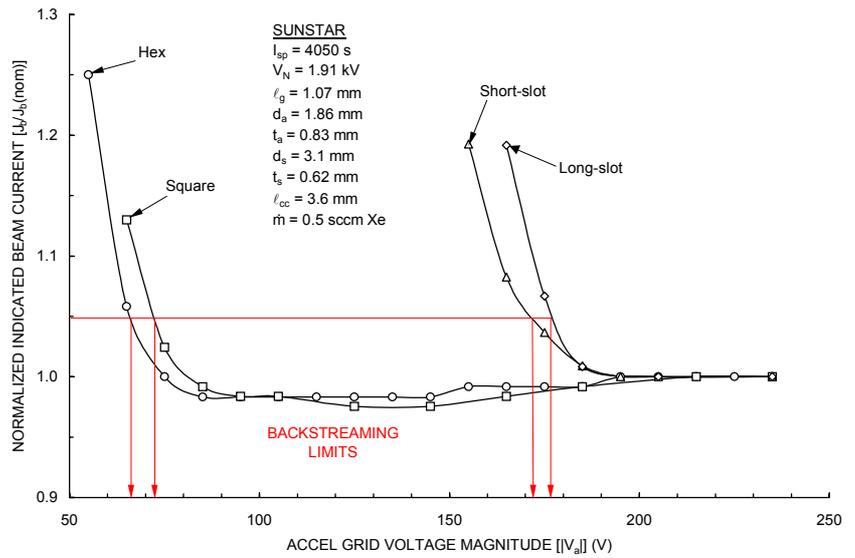
Fig. 4b Backstreaming limit data for the SUNSTAR gridlets throttled from 3000 to 6000 s.
