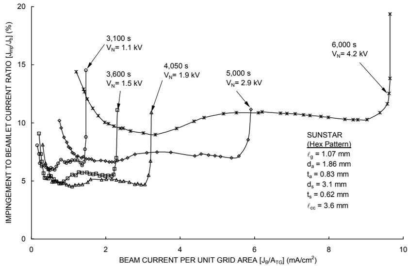
Fig. 5a Typical impingement current behavior for the hex pattern SUNSTAR gridlet versus specific impulse.
