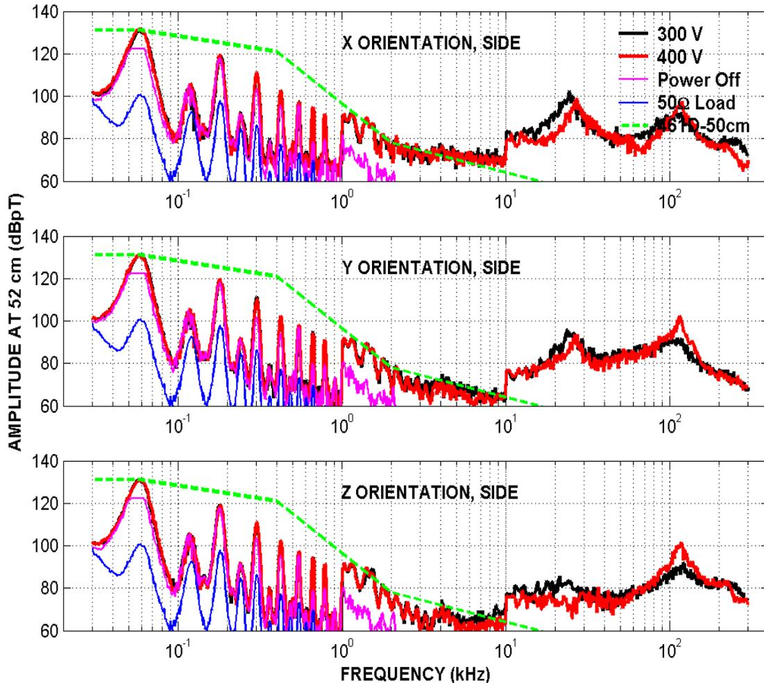
**Figure 7.** AC magnetic field at 52 cm to the side of the BPT-4000 operating at 4.5 kW. Orientations: X = coil axis horizontal and normal to thruster axis; Y = coil axis horizontal and parallel to thruster axis; Z = coil axis vertical.
