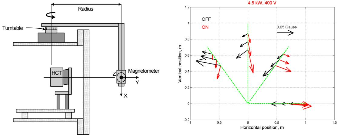
**Figure 8.** (a) Magnetometer setup shown with probe at 180° from thruster centerline and (b) plot of field for discharge off (magnetic field on) and discharge on.
