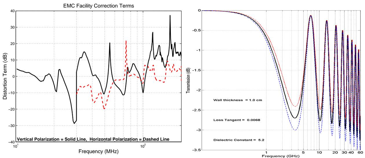
**Figure 2.** EMC anechoic room correction terms for vertical and horizontally polarized receiving antennas (left) and calculated transmission of fiberglass chamber (right).
