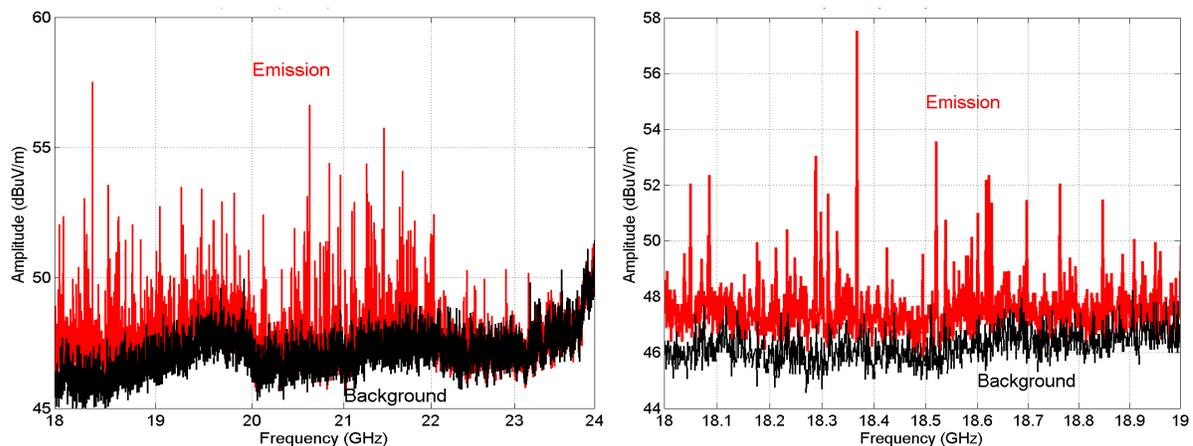
**Figure 6.** Expanded views of horizontally polarized emission spectra from BPT-4000 operating at 4.5 kW and 400 V.
