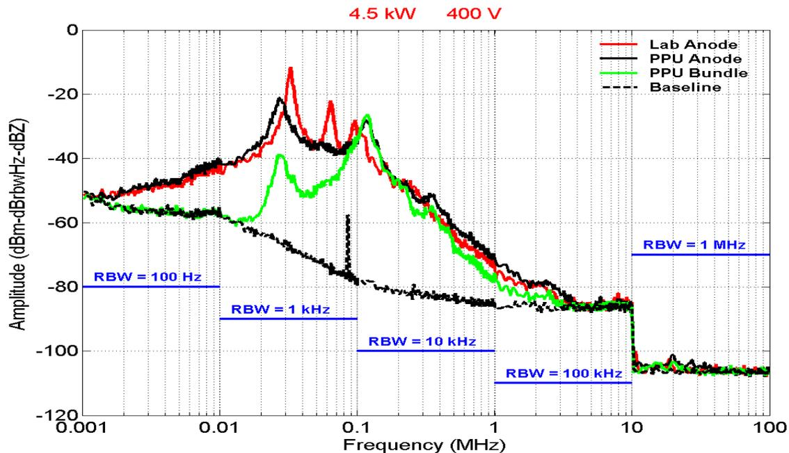
**Figure 10.** Spectra of current oscillations (4.5 kW, 400 V). The resolution bandwidths (RBW) are indicated.
