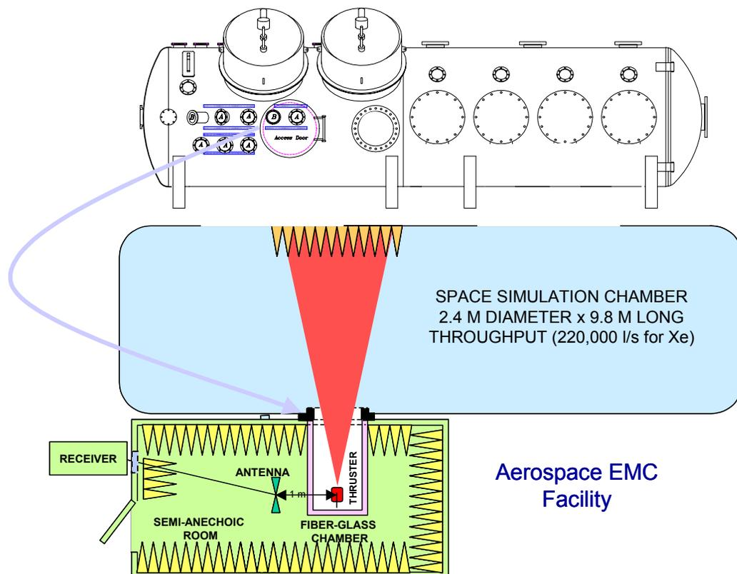
**Figure 1.** Layout of the facility used to measure electromagnetic emissions from the BPT-4000 thruster.
