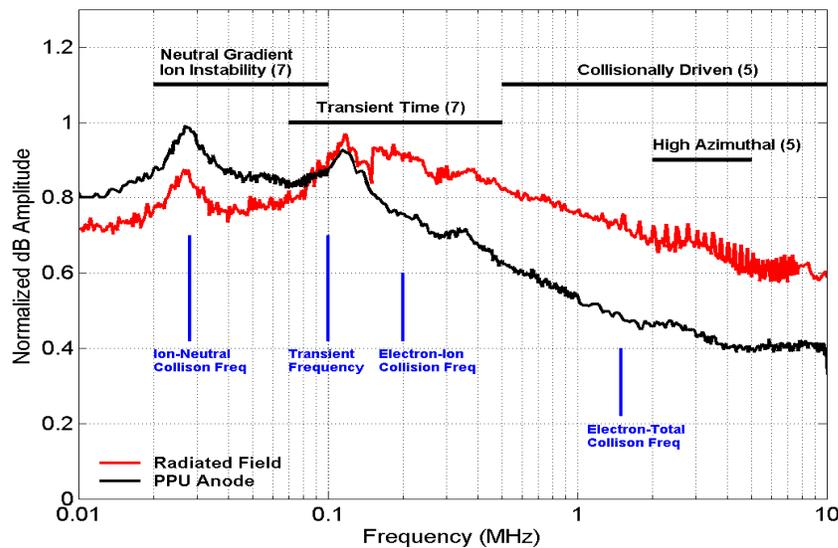
**Figure 11.** Spectra of current oscillations at 4.5 kW and 400 V.
