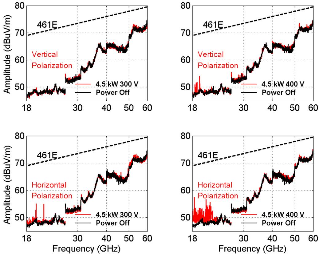
**Figure 5.** Vertically and horizontally polarized emission from BPT-4000 operating at 4.5 kW between 18 and 60 GHz.
