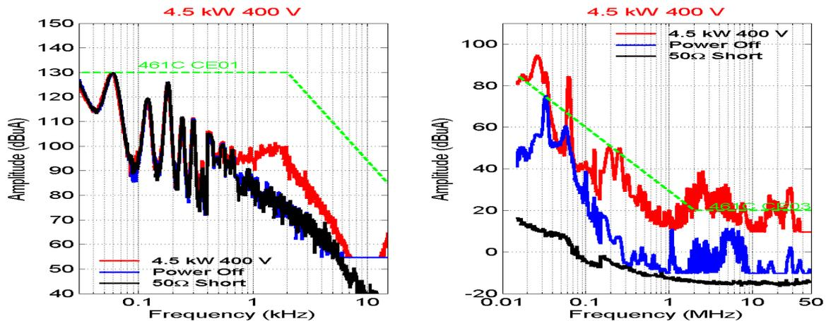
**Figure 9.** CE01 and CE03 conducted emissions for 4.5 kW and 400 V.
