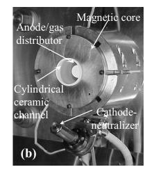
Fig. 2. (a) The 9 cm and (b) the 2.6 cm cylindrical Hall thrusters.
