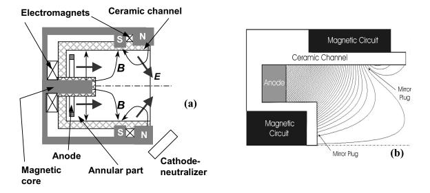
Fig. 1 (a) Schematic of a cylindrical Hall thruster. (b) Typical magnetic field distribution in a CHT.
