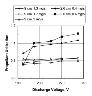
Fig. 3 Propellant utilization coefficient in the 9 cm and 2.6 cm cylindrical Hall thrusters. [From Ref.'s 6,7].
