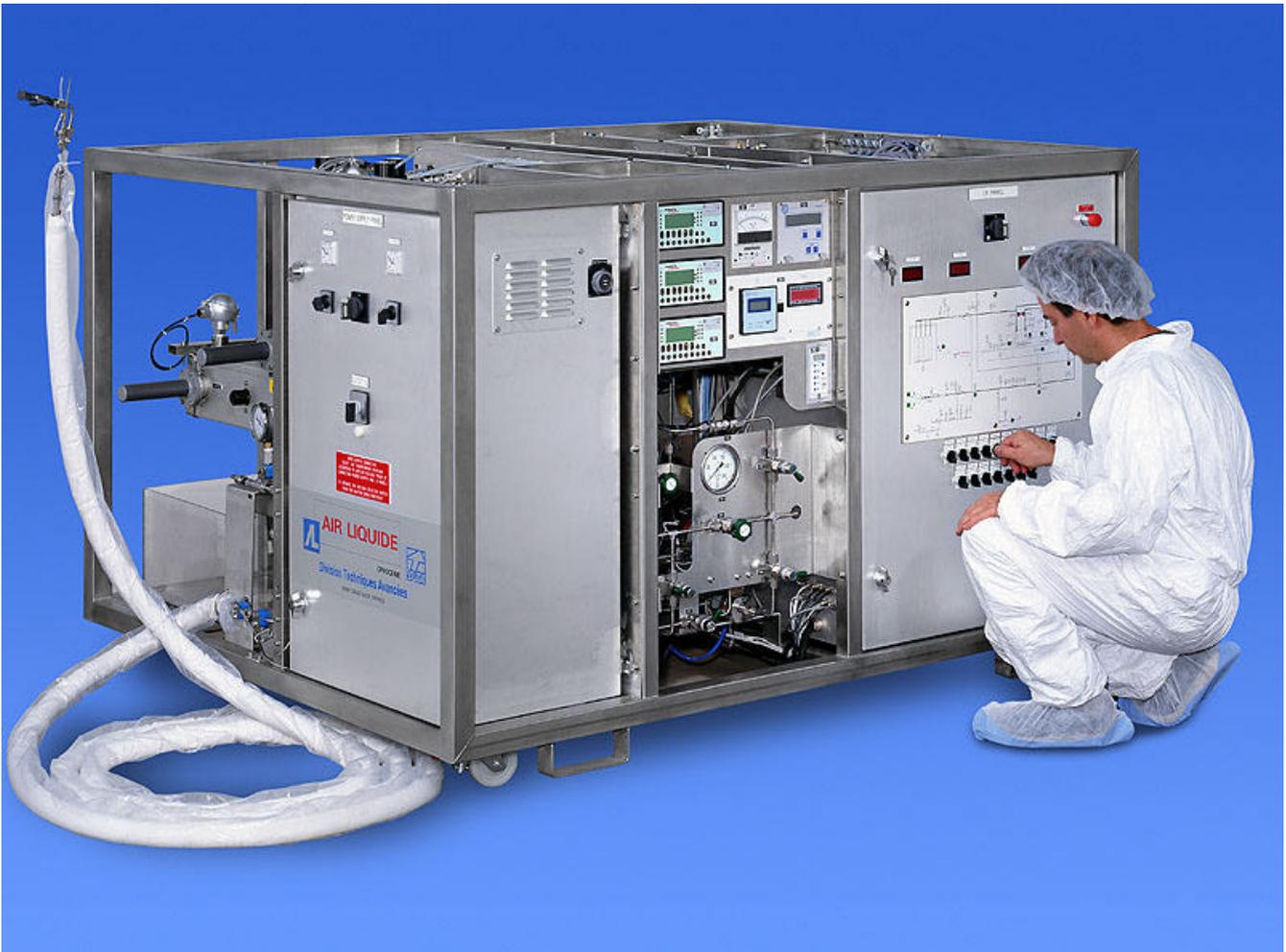
**Figure 1 : photo of the AIR LIQUIDE Xenon Ground Supply Equipment**
