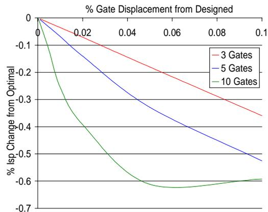
**Fig. 13. Isp change due to gate spacing**
