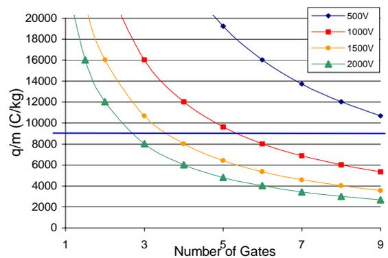
Fig. 6. Charge-to-mass ratio required for  $I_{SP}=1000s$  and  $X_{G1}=1mm$ . 9000 C/kg is an expected operational target
