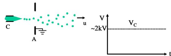
**Fig. 3. Schematic of a typical colloid engine and extraction voltage.**
