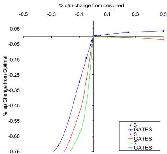
**Fig. 10. Isp change due to q/m for a single particle**
