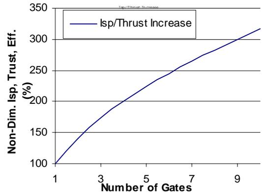
Fig. 5. Performance increase due to multiple gates versus single accelerator gate. Assumes constant extraction parameters and gate voltages.
