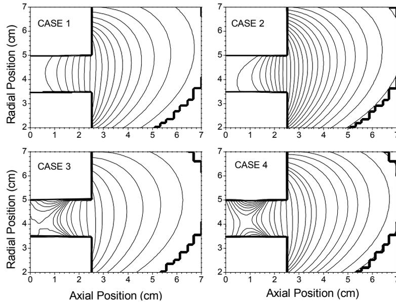
Figure 1 : SPT100 magnetic field lines calculated with FEMM for 4 different configurations of the magnetic circuit. The channel is located on the left-hand side of the plots between the radial positions 3.45 and 5 cm ; the exhaust is at an axial position of 2.5 cm.
