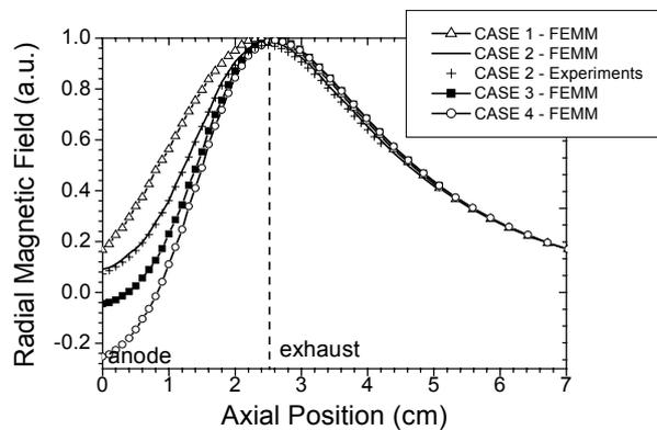
Figure 2 : Axial variations of the calculated radial magnetic field strength at the thruster channel median for different configurations. Measurements for the SPT100-ML are also plotted for CASE 2.
