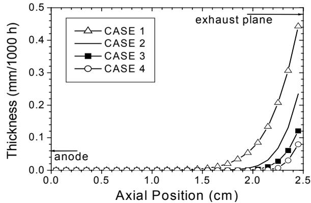
Figure 4 : Calculated erosion rate of the inner channel wall.
