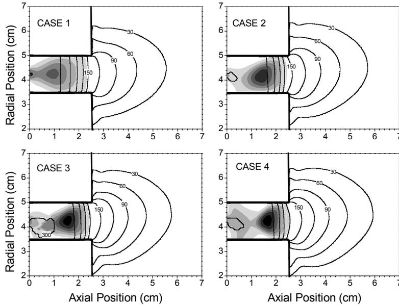
Figure 3 : Time-averaged spatial profiles of the electric potential (contours) and the ionization source term (gray scale). The contours are equally spaced with intervals of 30 V. The gray scale is linear, the intervals correspond to  $10^{23} \text{ m}^{-3} \text{ s}^{-1}$ .
