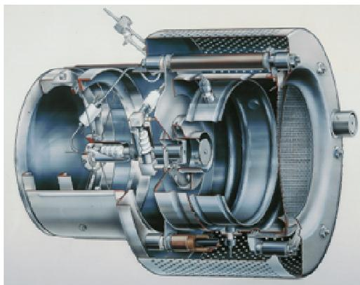
*Figure 11. Artist's impression of a sectional view of the T5 Mk 1 thruster.*
