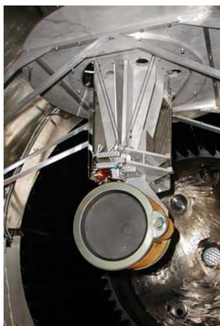
**Figure 19.** T6 thruster mounted on thrust balance.
