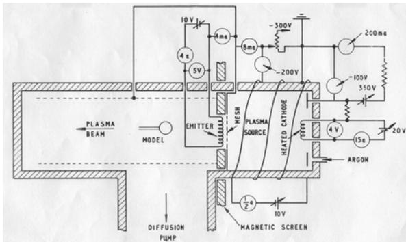
**Figure 1.** Ion source designed by at Fort Halstead.
