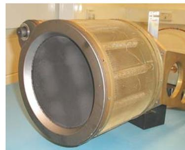
**Figure 16.** UK-25 25 cm beam diameter thruster. **Figure 17.** The T6 22 cm beam diameter thruster.
