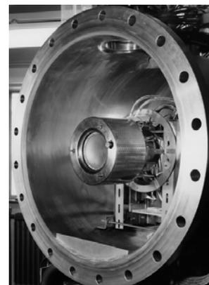
*Figure 12. T5 Mk 1 thruster in load-lock of RAE's test facility.*
