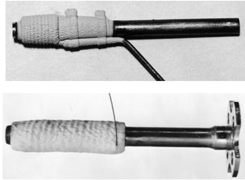
**Figure 6.** Hollow cathodes for the T2 thruster. Top: made by GEC. Bottom: made by RAE.
