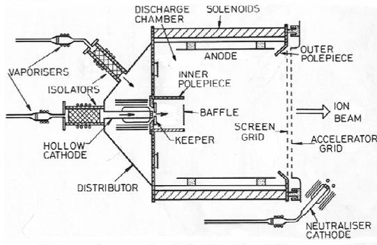
**Figure 5.** Sectional diagram of the T2 thruster.
