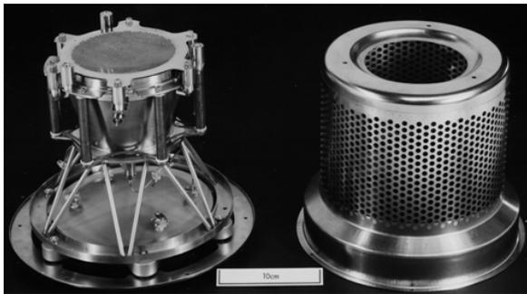
*Figure 9. Photo of T4 thruster.*
