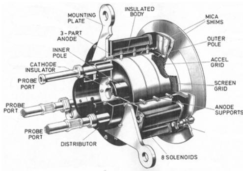
**Figure 7.** Sectional diagram of the Culham 15 cm thruster.
