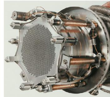
**Figure 14.** Summary of the performance of the T5 thruster. **Figure 15.** T5 Mk 4 thruster without earth screen.
