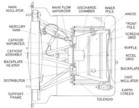
**Figure 8.** Sectional diagram of the T4 thruster.
