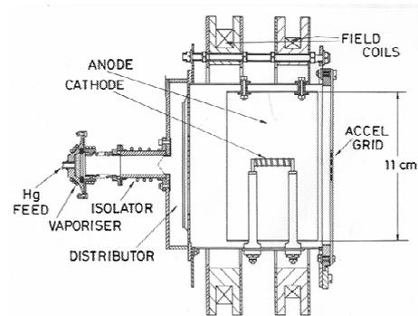
**Figure 2.** The initial configuration of T1 thruster.
