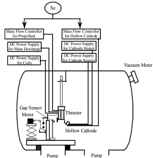
Figure 3 Schematic view of test facility.
