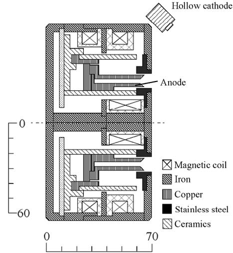
Figure 1 Cross-sectional view of TALT-2 Hall thruster without magnetic shields.
