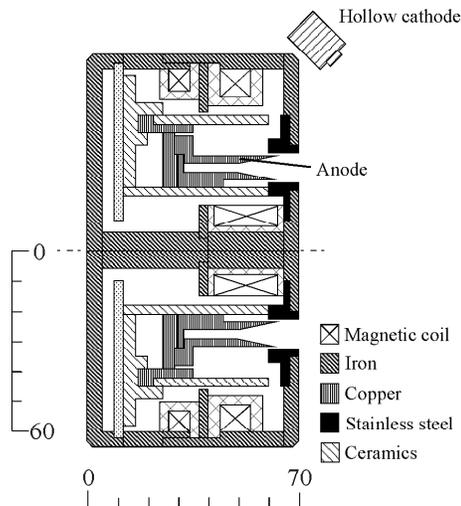
**Figure 10 Cross-sectional view of new TALT-2 Hall thruster with unique hollow anode.**
