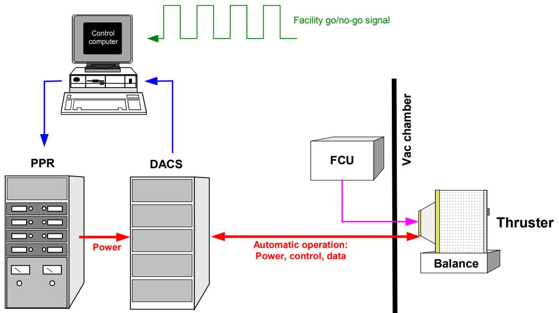
**Figure 9 Electrical Power and Data Acquisition Architecture**
