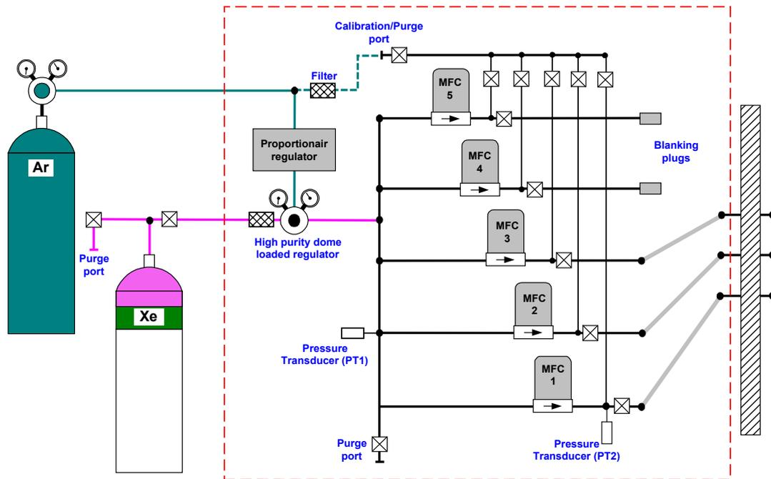
**Figure 8 Propellant Feed System**
