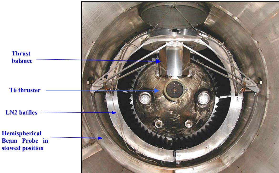
**Figure 7 Photograph of the ion beam probe array within the 3.8m vacuum facility**
