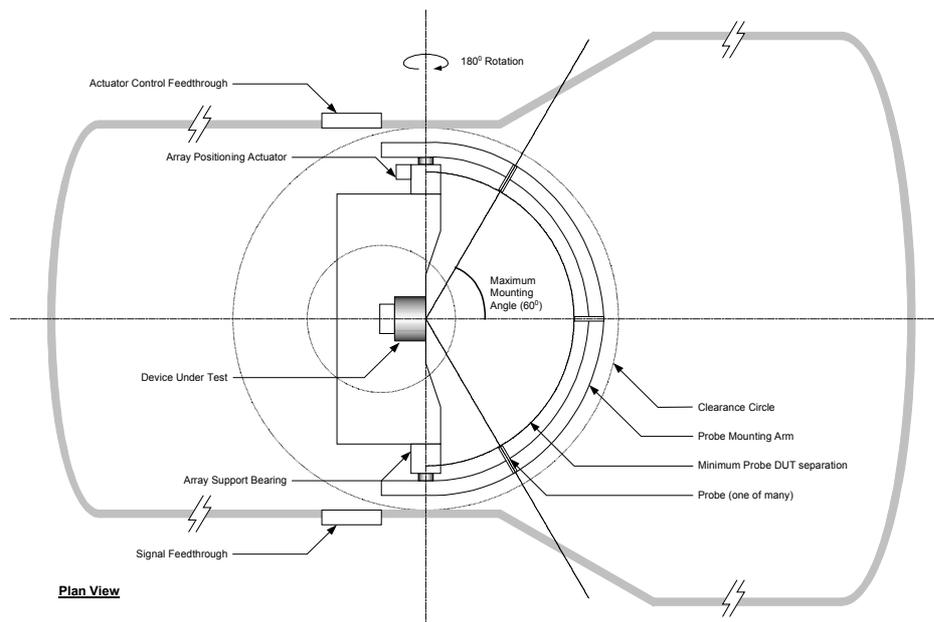
**Figure 6 Schematic of large diameter ion beam probe array**
