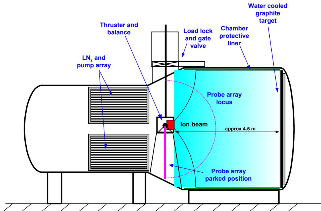
**Figure 1 Schematic of LEEP2 Test Facility**
