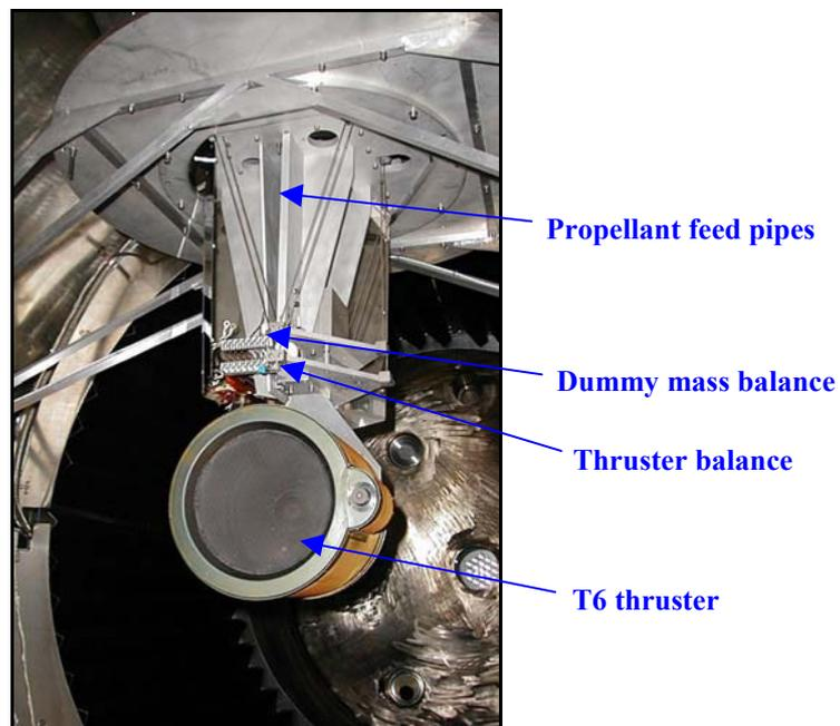
**Figure 5 Photograph of the thrust balance with a T6 thruster fitted**
