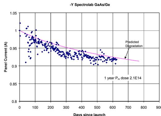
**Figure 5** Degradation of STRV-1b GaAs/Ge solar panel in GTO.
