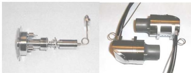
**Figure 2** Photographs of QinetiQ hollow cathodes.
