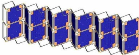
**Figure 4** Partially deployed QinetiQ hybrid solar array.
