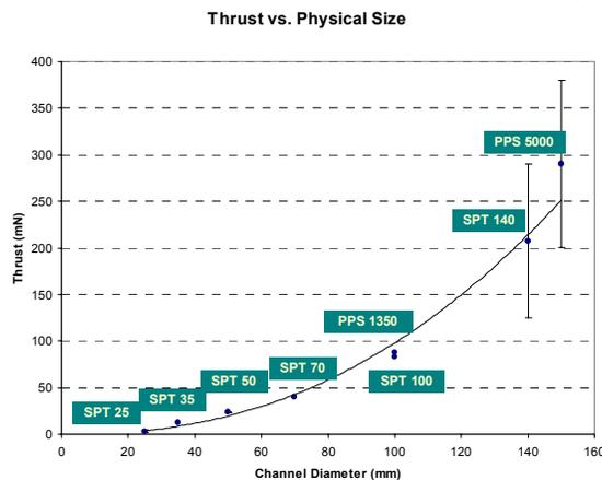
**Figure 1** Thrust as a function of physical size for selected SPTs.
