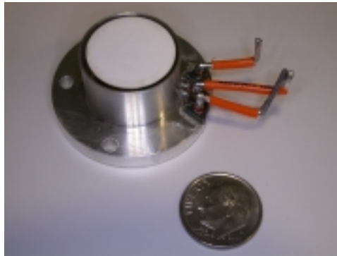
Figure 4 – Generic Radiometer Design for Contamination Measurements
