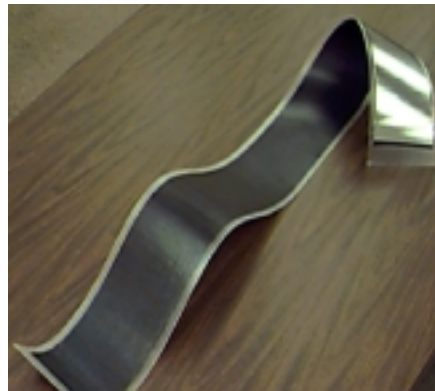
Figure 5 – Thin-Film Solar Array Technology Similar to that used on the main array
