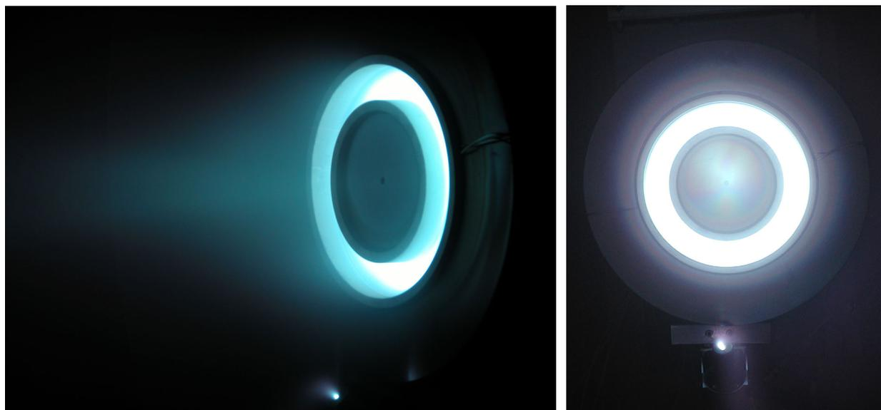
**Fig. 12 Thruster firing in Alta IV-4 facility.**
