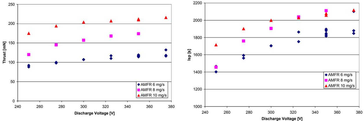
**Fig. 10 Thrust (left) and specific impulse (right) vs discharge voltage.**
