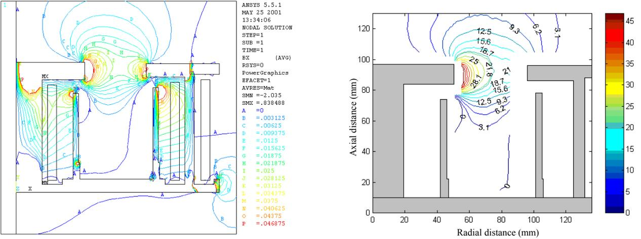
Fig. 6 Radial magnetic field component: numerical simulation (left) and experimental results (right).
