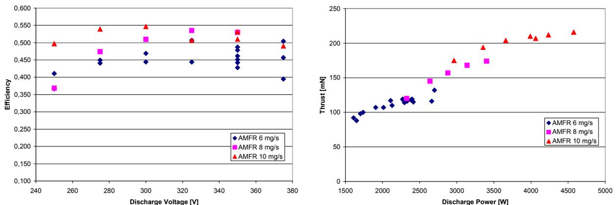
**Fig. 11 Efficiency vs discharge voltage (left), thrust vs discharge power (right)**
