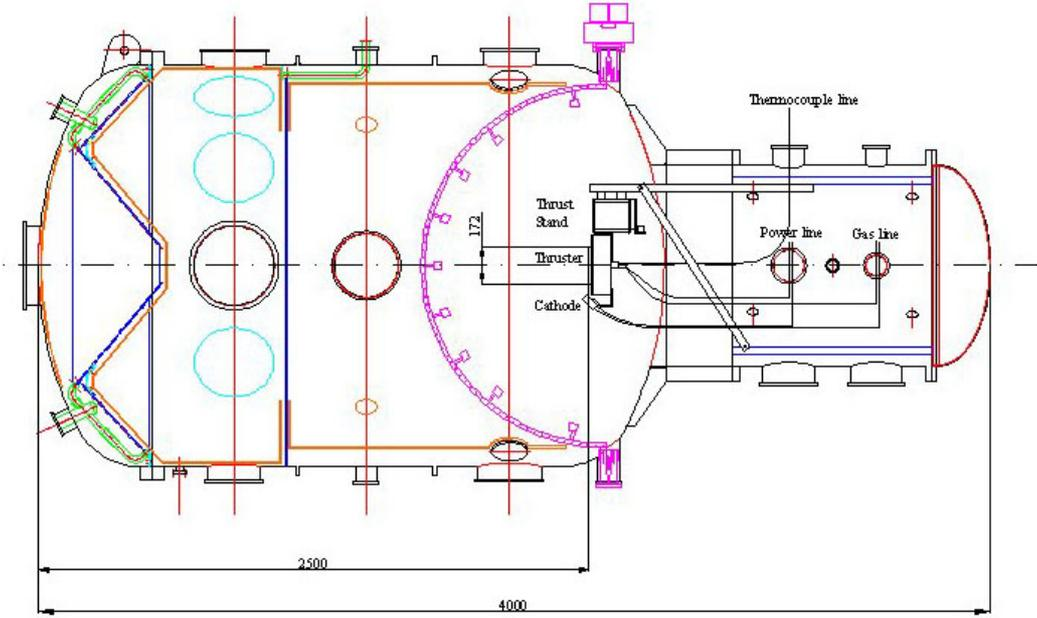
Fig. 5 Alta IV-4 test facility schematic.
