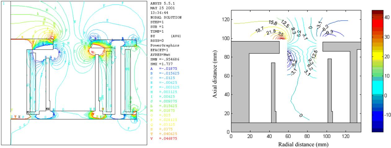
Fig. 7 Axial magnetic field component: numerical simulation (left) and experimental results (right).
