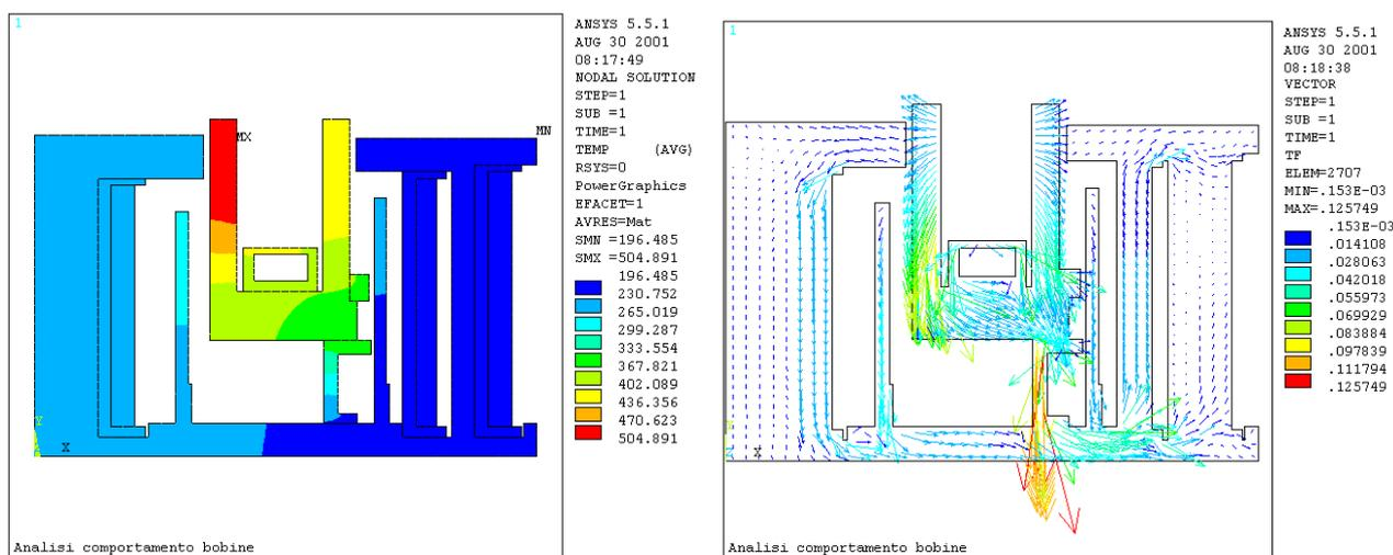
Fig. 4 Temperature and thermal flux distributions.
