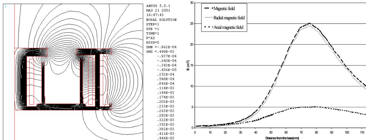
**Fig. 3 Magnetic induction lines distribution (left) and value of the magnetic induction components along the channel centreline.**
