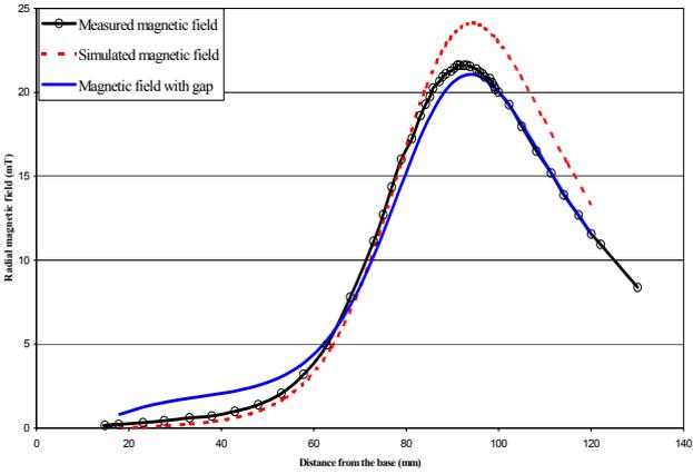
Fig. 8 Comparison between the simulated and measured radial magnetic field.
