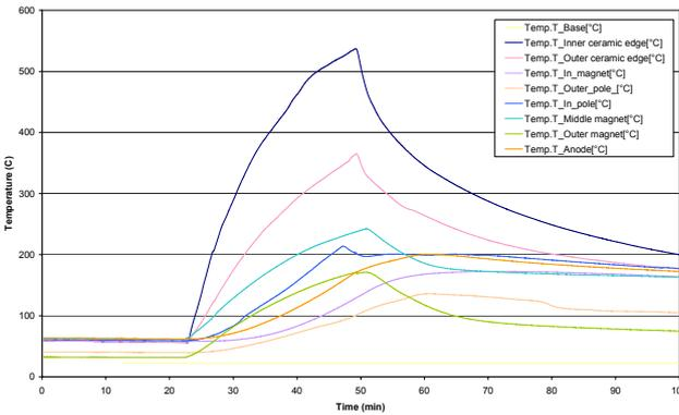
Fig. 9 Experimental temperature history in different positions, discharge power 3800 W, total power (discharge+magnets) 4250 W.
