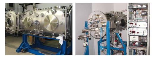
Fig. 9 - The FEEP lifetime and qualification test facility, left; one of three identical support test chambers, right.
