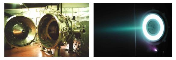
Fig. 14 - Alta's IV4 test facility: 2 m diameter, 3.2 m long, with an additional 1 m diameter, 1 m long lock chamber; a 1 m diameter gate valve connects the two. At right, Astrium's ROS-2000 HET fired in Alta's IV-4 facility.
