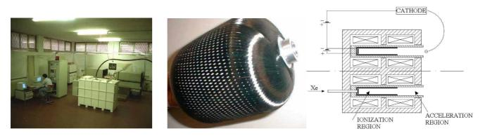
Fig. 5 - Low Energy Electron Accelerator for layer-by-layer composite curing, left; laboratory prototype of small tank prior to be submitted to electron irradiation for polymerization, middle; conceptual scheme of the proposed double stage Hall thruster, right.
