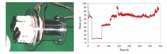
Fig. 8 - A twin-emitter FEEP cluster, left; thrust profile over 340 hours, right.
