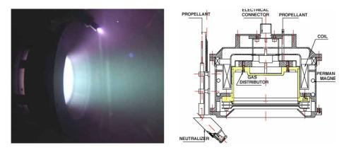
Fig. 1 - RMT Ion Thruster: under test at LABEN/Proel, left; cross section drawing, right.
