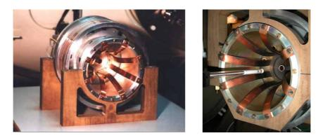
Fig. 10 - Centrospazio's HPT prototype: on the bench, left; with a magnetic probe assembly, right.
