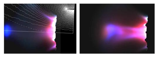
Fig. 12 - Picture of the HPT plume with calculated superimposed applied magnetic field, left; a plasma "clot" after expulsion, right.
