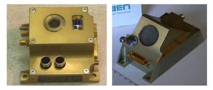
Fig. 3 -Ion Propulsion Diagnostic Sensor for ARTEMIS, left; Plasma Probe Assembly for STENTOR and SMART-1, right.
