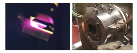
Fig. 7 - Rb-fed FEEP thruster plume, left; 100 µN thruster module, right.
