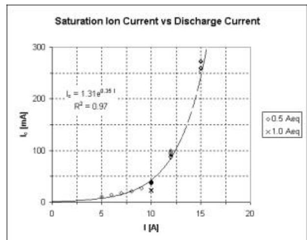
**Figure 2** – Saturation collected ion current.
