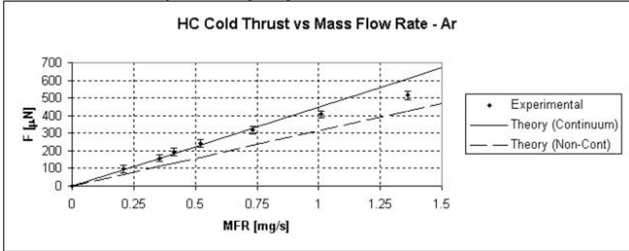
**Figure 3** – HC cold thrust (no discharge, no heating) vs mass flow rate.
