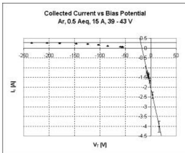
**Figure 1** – Target V-I characteristic.
