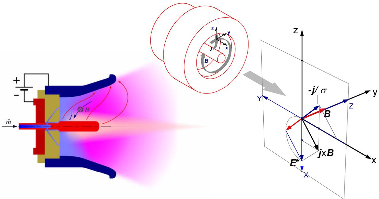
**Fig. 3 General scheme of self-field MPD thruster**
