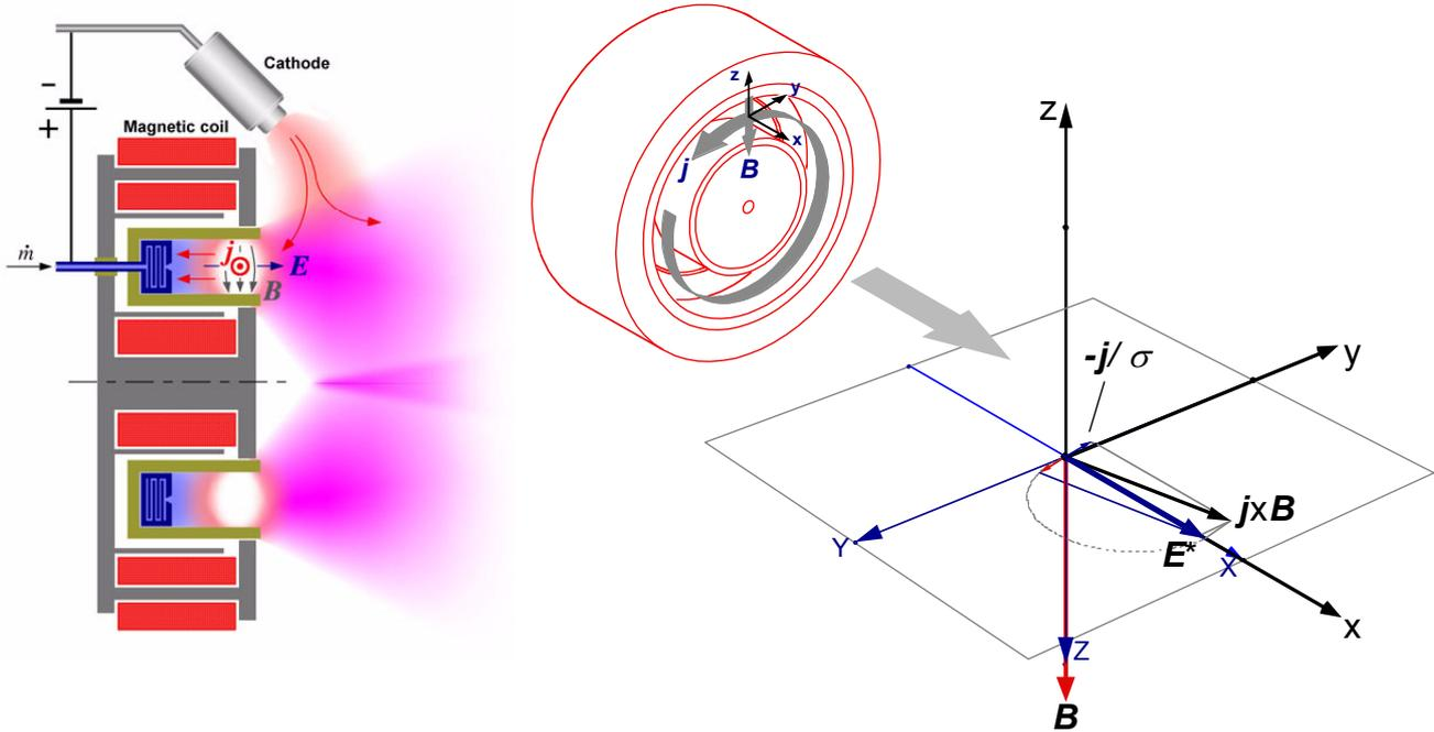
Fig. 2 General scheme of Hall effect thruster
