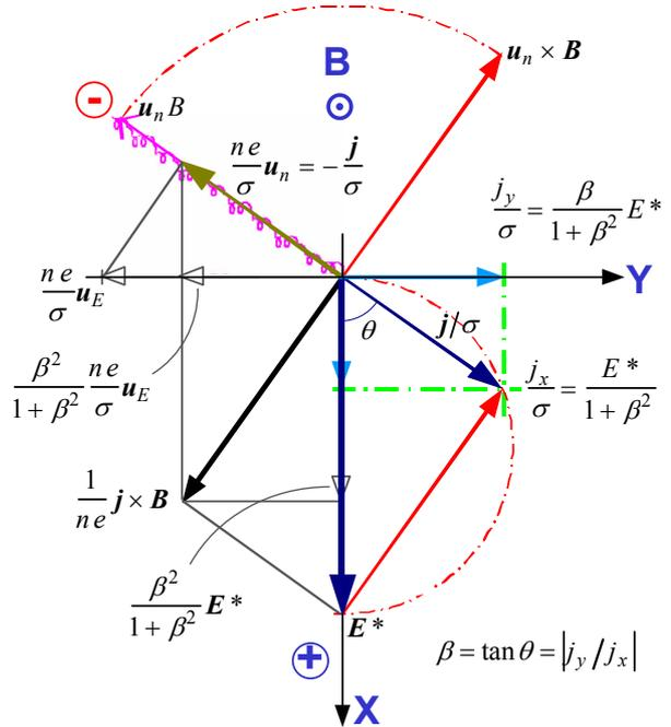
**Fig. 1 Vector diagram for fields and currents in plasma thrusters**
