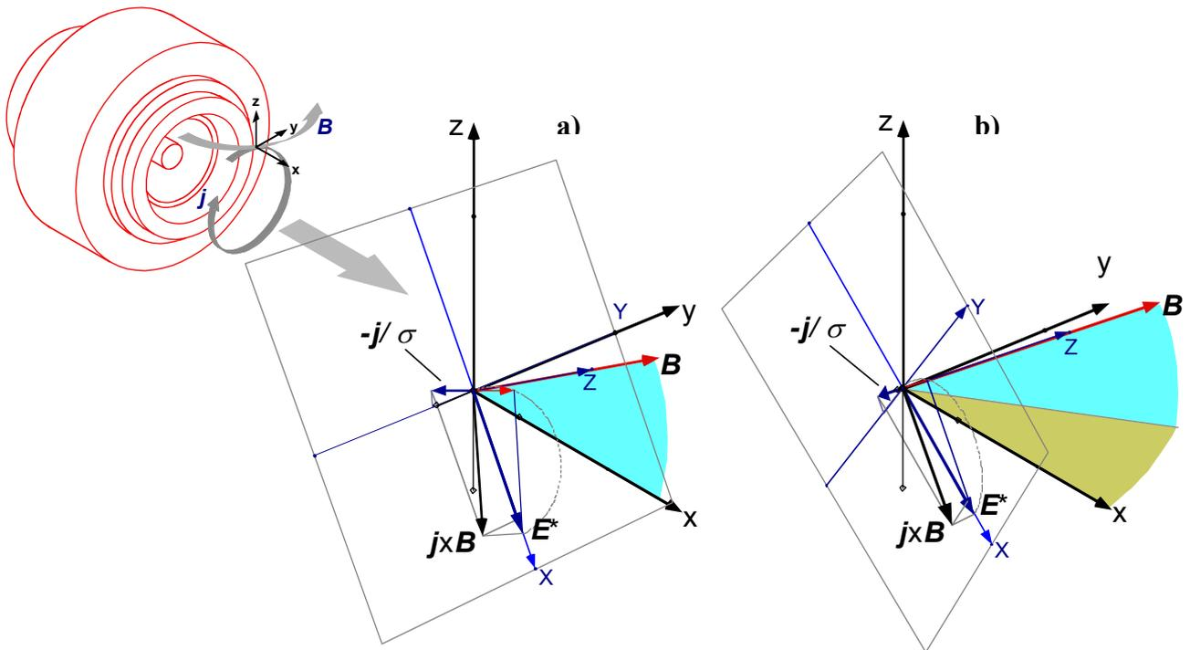
Fig. 5 Vector diagrams for applied-field MPD thruster
