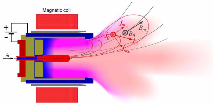
Fig. 4 General scheme of applied-field MPD thruster
