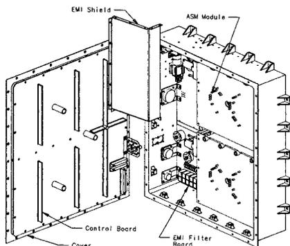
Figure 6 – HTPS PPU Mechanical Design
