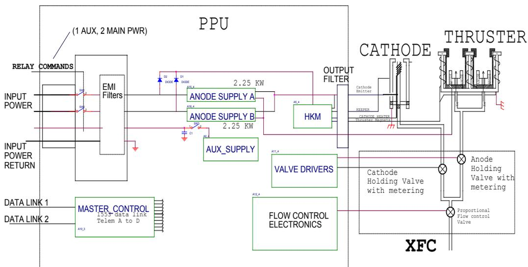
Figure 5 – HTPS PPU Block Diagram
