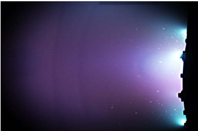
Fig. 15: Plasma plume in regime conditions registered with t_{exp} = 5 \mu s and t_d = 1 ms.
