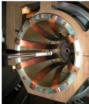
Fig. 5: A single three-axes magnetic probe (a), and the magnetic system probes in the thruster (b).
