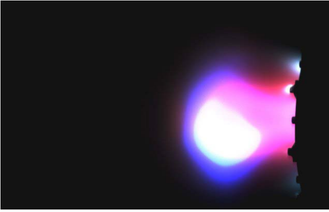
Fig. 17: Plasma "clot" during the expulsion from thruster with t_{exp} = 10 \mu s and delay t_d = 25 \mu s .
