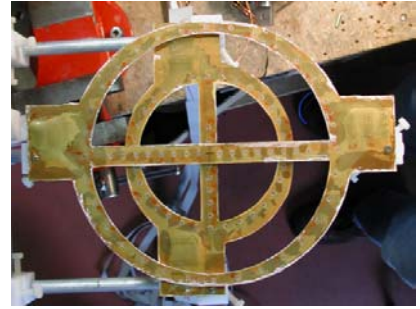
Fig. 4: The assembled annular system of electrostatic probes, before the deposition of the Boron-Nitride film.
