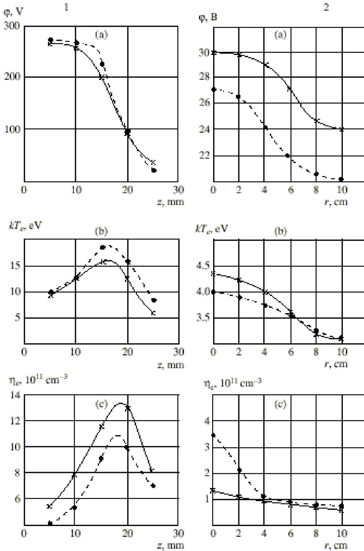
**Fig. 3.** Distributions of the plasma potential (a), electron temperature (b), and electron density (c) in the channel (I) and in the jet (II) behind the outlet of the accelerator at  $\dot{m} = 2 \text{ mg/s}$  and  $U_d = 300 \text{ V}$  for Kr (crosses) and Xe (circles); the anode and the accelerator outlet are located at  $z = 0$  and  $25 \text{ mm}$ , respectively.
