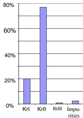
Fig. 6. Radiation Energy Distribution onto Particles in Ionization Region of A-3 Channel on Kr
