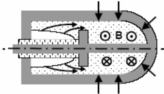
Figure 2. Schematic arrangement<sup>16</sup> of MAGO configuration<sup>11</sup> in which an inverse-pinch discharge pushes plasma magnetized with azimuthal field into an implosion chamber. The azimuthal field provides thermal insulation for plasma supported by walls.
