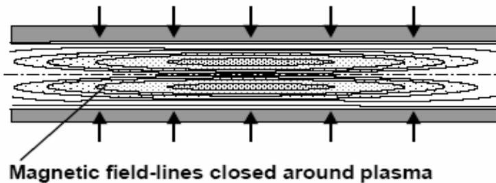
Figure 4. Field-reversed configuration (aka, *compact toroid*) within imploding liner provides distribution of closed-field lines containing plasma, for both thermal insulation and mechanical support<sup>16</sup>.
