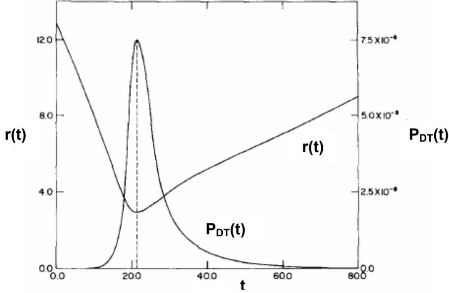
**Figure 6. Calculated<sup>18</sup> trajectory of inner surface of liner and D-T reaction rate  $\underline{vs}$  time for a case of substantial liner material-compression ( $\zeta = 0.794$ ), displaying asymmetry of trajectory around minimum radius due to liner compressibility**
