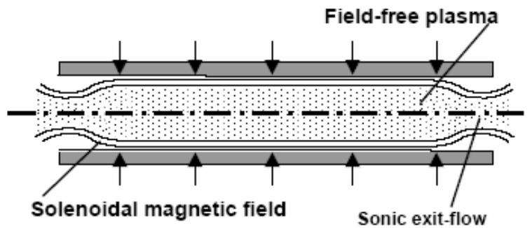
Figure 3. “Theta-pinch-with-liner” concept<sup>16</sup> for imploding liner compression of plasma to fusion conditions. (Magnetic “nozzles” that occur at open ends due to supersonic flow to vacuum are not MHD stable.)
