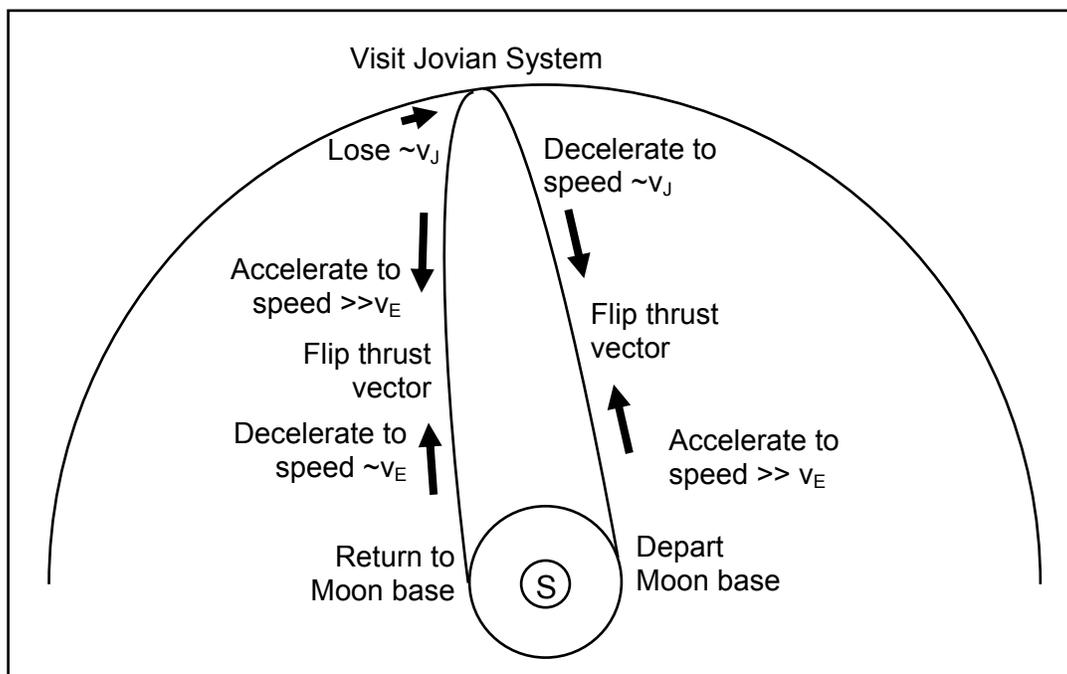
**Figure 1. Sketch of fast mission to Jovian System in which continual acceleration or deceleration supplies effective gravity for the crew. Cargo of equipment and propellant precedes mission by more efficient, slower trajectory.**
