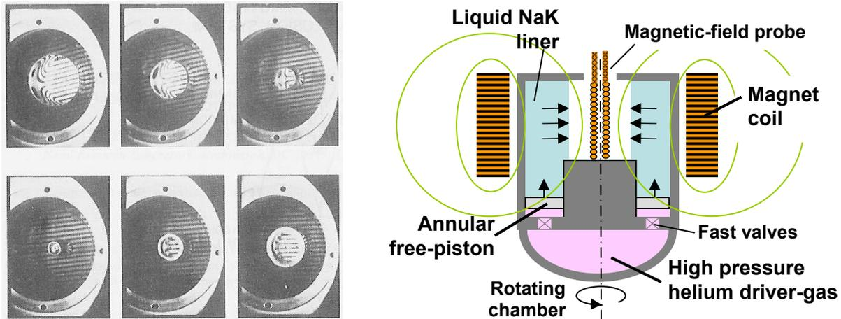
Figure 5. Frames from high-speed movie of stabilized liner implosion and re-expansion in hydrodynamic experiments<sup>2</sup>. The liner material here is water and the free-piston pneumatic power system uses high pressure air. The liner and its chamber rotate to prevent Rayleigh-Taylor instability of the inner surface as it compresses trapped air. Similar experiments were performed with liners of NaK, driven by helium and compressing argon and magnetic flux, shown schematically on the right.
