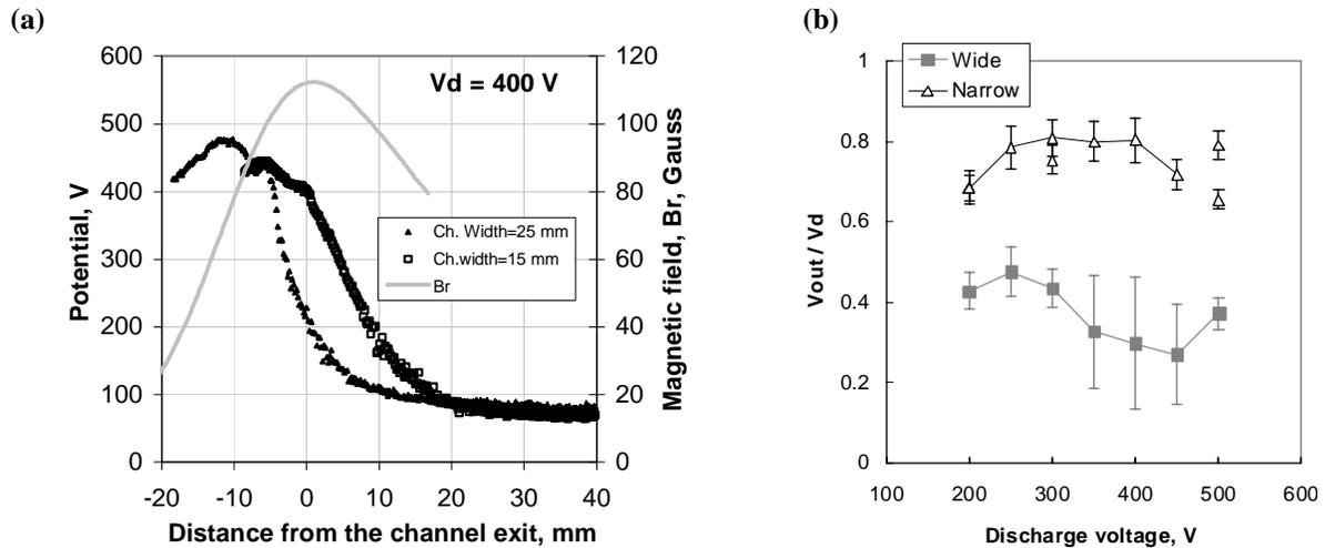
Figure 2. Plasma measurements for two thruster configurations with different boron nitride channels of 25 mm width and 15 mm width: the plasma potential distributions for the discharge voltage of 400 V (a); the outside voltage drop in the near-field plasma plume,  $V_{out}$ , as a function of the discharge voltage,  $V_d$  (b).<sup>8</sup> Magnetic field is not changed with the discharge voltage.
