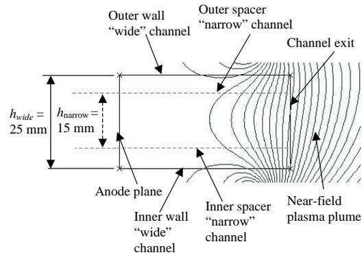
**Figure 1. Schematic of the thruster channel for two different channel widths (15 mm and 25 mm) with superimposed magnetic field lines.<sup>8</sup>**
