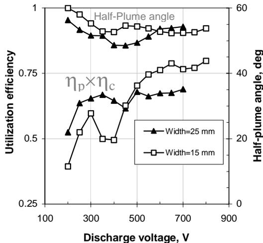
Figure 3. Results of plume measurements for two thruster configurations with two different channel widths: 25 mm and 15 mm. Propellant utilization times current utilization<sup>8</sup> and half-plume angle obtained for 90% of the total ion flux. Magnetic field is not changed.
