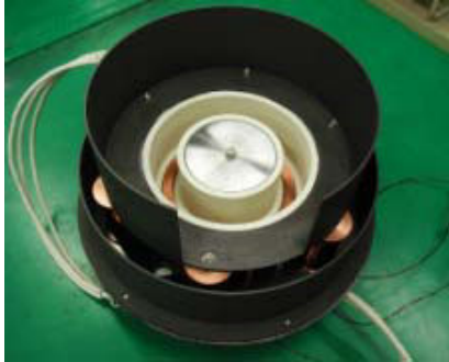
Figure 6. Accelerator DM with plume shield.
