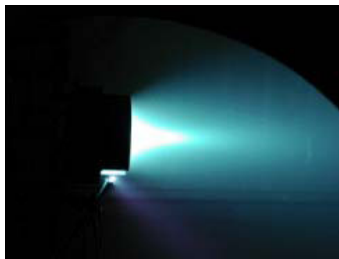
Figure 18. Hall Thruster DM is on operation.
