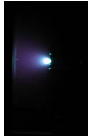
Figure 12. Photograph of the hollow cathode on operation.
