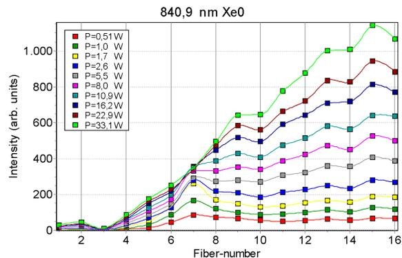
Figure 12. Intensity versus fiber position, result of position sensitive Emission Spectroscopy. (pos 3 center of electrode, pos 16 cylinder center)
