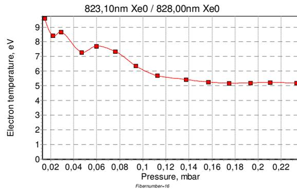
Figure 11. Electron temperature as a function of inner pressure measured by Emission spectroscopy on center axis.
