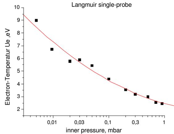
Figure 10. Electron temperature as a function of inner pressure measured by Langmuir-single-probe on center axis.
