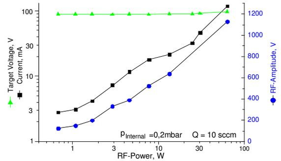
Figure 8. Extracted electron current, RF-amplitude and target voltage as function of RF-power
