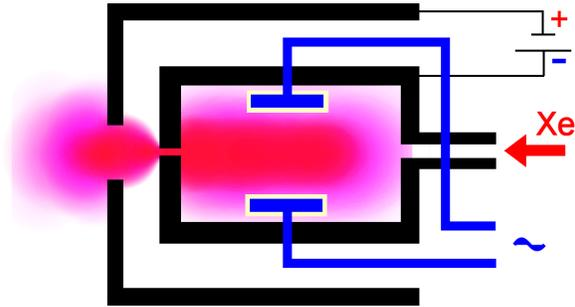
Figure 1. Principle of capacitive neutralizer – the insert has been replaced by RF-electrodes
