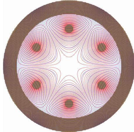
**Figure 3. Simulated electric equipotential lines (red) and magnetic field-lines (blue)**
