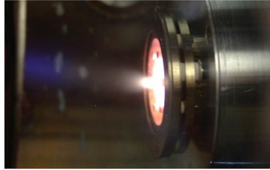
Figure 7. Neutralizer in operation (with mica diaphragm)
