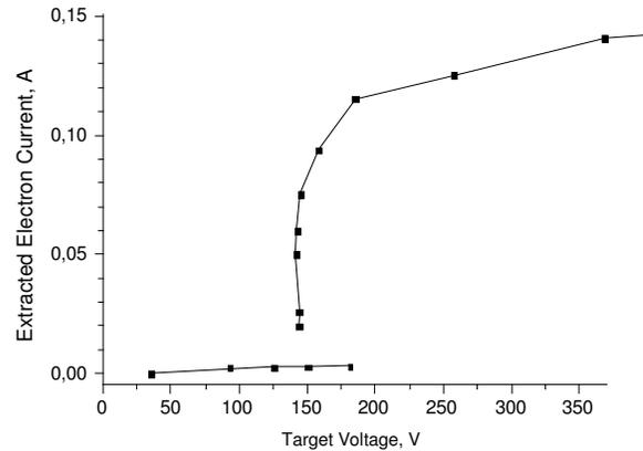
**Figure 13. Extracted electron current as function of target voltage.**
