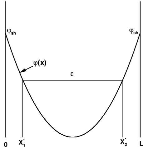
Figure 2. Schematic of electron potential energy profile  $\phi(x)$  in the plasma slab, due to the electrostatic field. An electron with total ( $x$ -kinetic plus potential) energy  $\epsilon$  will reflect back at points  $x_1^*$  and  $x_2^*$  (turning points).
