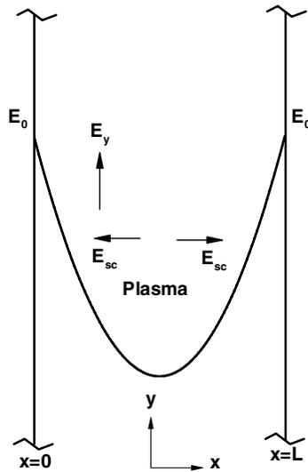
**Figure 1. Schematic of a one-dimensional plasma slab of length  $L$  powered by a symmetric coupled source. The RF current source (not shown) results in an RF field in the transverse direction,  $E_y$ . The value of the field at the edges,  $E_0$ , is determined by the desired power deposition in the plasma. A space charge field  $E_{sc}$  develops in the  $x$ -direction to confine electrons.**
