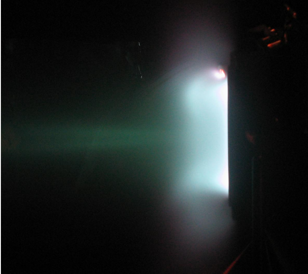
Figure 40. Image of operating thruster, showing plume “jet” and slight asymmetry associated with cathode.
