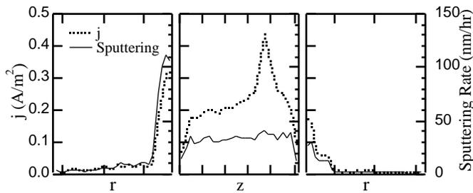
Figure 11. Current density and Sputtering rate on Ac grid
