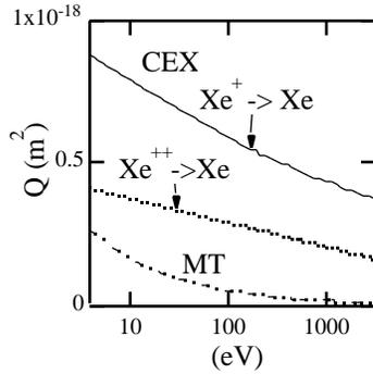
Figure 6. Collision cross section<sup>9,10</sup>
