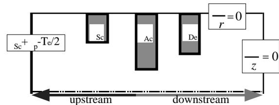
Figure 3. Boundary conditions for electric potential
