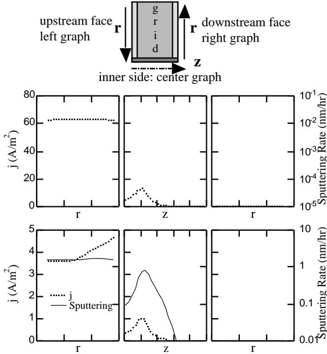
Figure 10. Current density and Sputtering rate on Sc grid (Upper: Singly charged, Lower: doubly-charged)
