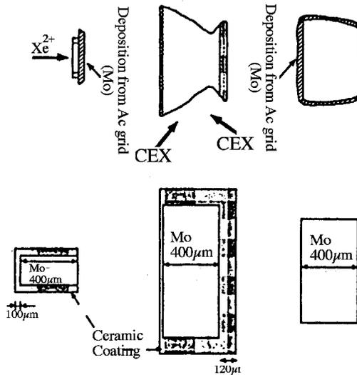
Figure 14. Sectional shape of the ETS-6 grid after the endurance test (initial: below, after 7,000 hours operation: above).
