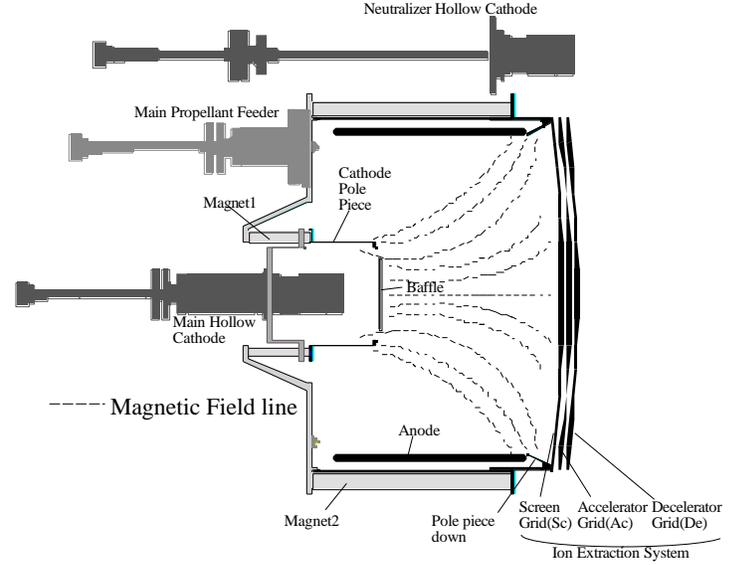
Figure 1. The schematic diagram of the Kaufman-type ion thruster.
