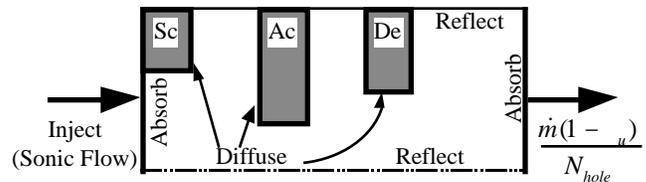
Figure 5. Boundary conditions for neutral particles
