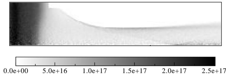
Figure 9. Ion number density (m<sup>-3</sup>)
