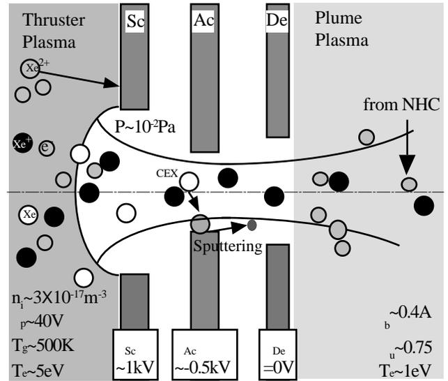
Figure 2. Ion extraction and sputtering model of beam extraction system.
