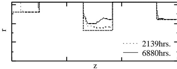
Figure 13. Calculated grid shape change in the ETS-6
