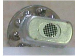
Figure 10. CNT cathode with mesh gate.
