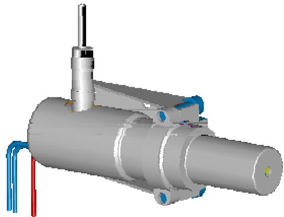
Figure 8, Neutralizer Cathode
