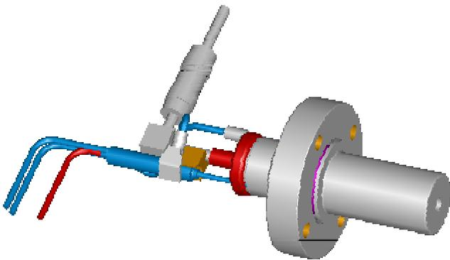
Figure 7, Discharge Cathode
