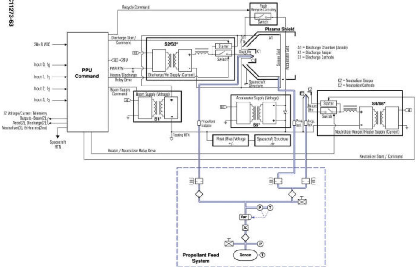
Figure 5, Low Power Ion Propulsion System Block Diagram
