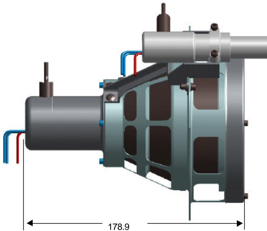
Figure 4, Low Power Ion Thruster, Side View
