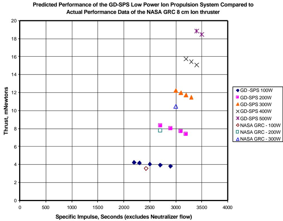
Figure 6, Predicted Low Power Ion Propulsion System Performance
