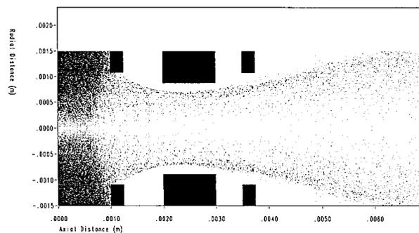
Figure 14 – Computed ion distribution within the grids
