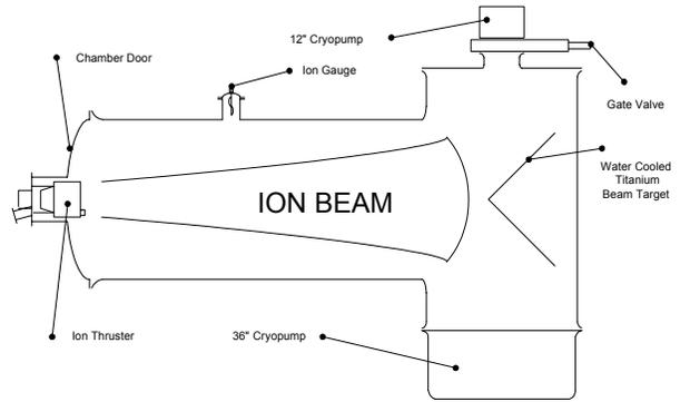
Figure 3 – Schematic diagram of the smaller QinetiQ test facility.
