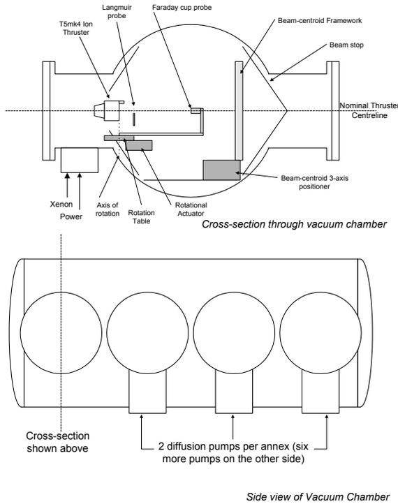
Figure 2 – Schematic diagram of the Aerospace Corporation test facility.
