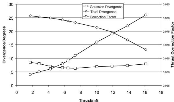
Figure 13 – Ion beam divergence for the two analysis techniques and thrust correction factor as functions of thrust.
