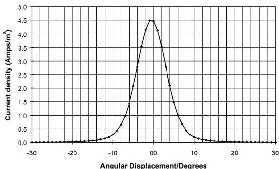
Figure 8 – Ion beam profile from the Aerospace Corporation Faraday cup probe at 10 mN thrust.
