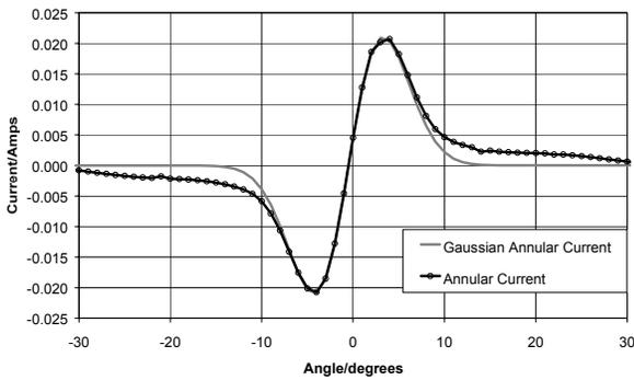
Figure 11 – Comparison between experimental annular ion current and that assumed in a Gaussian approximation.
