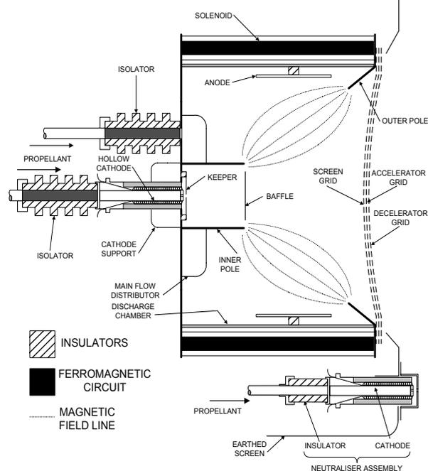
Figure 1 – Schematic cross sectional view of the T5 ion thruster.
