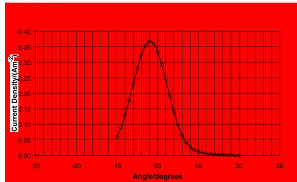
Figure 9 – Ion beam profile from the QinetiQ Faraday cup probe at 10 mN thrust.
