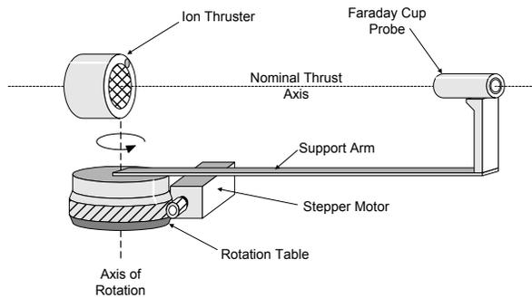
Figure 5 – Mounting arrangement for the Aerospace Corporation Faraday cup probe.
