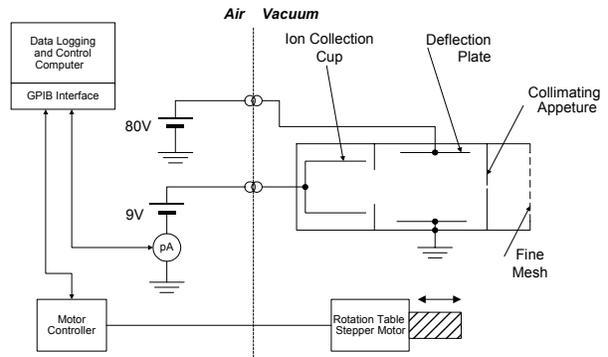
Figure 4 – Schematic diagram of the Aerospace Corporation Faraday cup probe.
