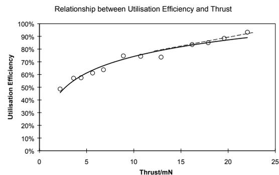
Figure 7 – Propellant utilisation efficiency as a function of thrust.
