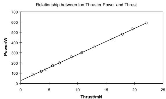
Figure 6 – Power consumption as a function of thrust.
