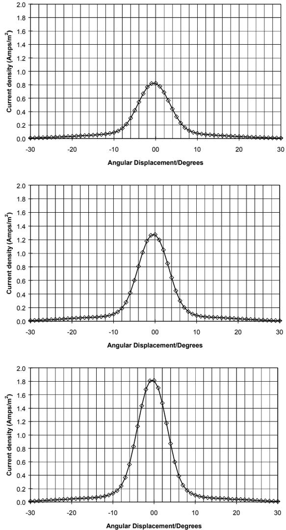
Figure 12 – Ion beam profile from the Aerospace Corporation probe at 3.7 mN (top), 4.7 mN (centre) and 5.7 mN (bottom) thrust.
