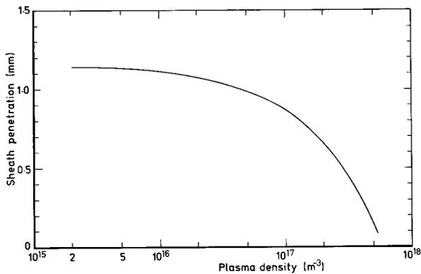
Figure 17 – Sheath penetration into the discharge chamber plasma as a function of  $n_e$ .
