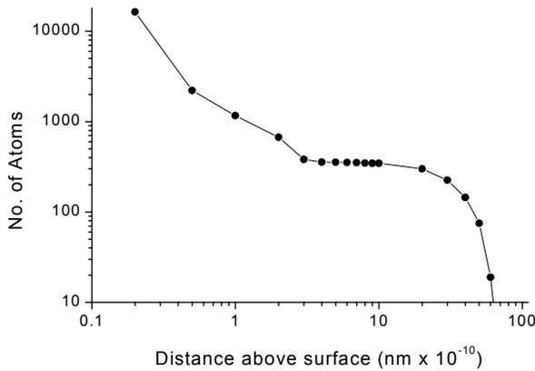
Figure 2 - Distribution of Mo atoms above the surface for a Mo(110) target bombarded with 500 eV Xe ions.
