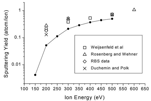
Figure 5 – Sputtering yield of molybdenum as a function of xenon ion energy. Results obtained from computer simulation are presented as solid circles.
