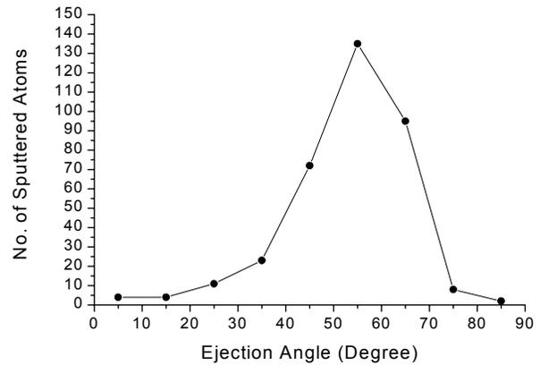
Figure 4 – Number of sputtered atoms as a function of ejection angle.
