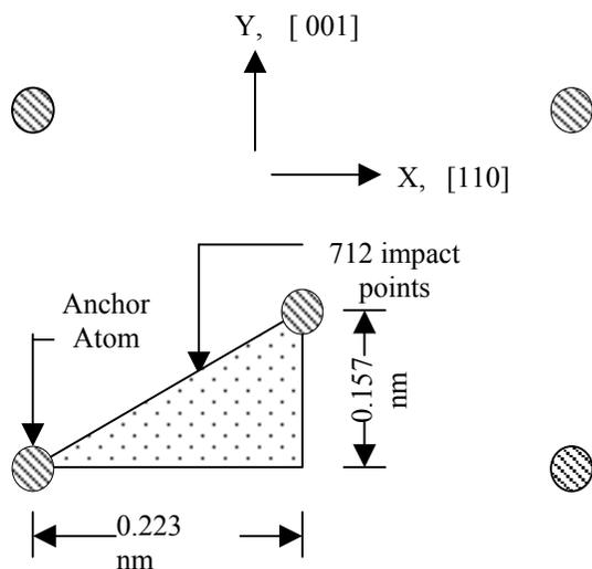
Figure 1 – Projectile impact zone. The target surface lies in the (110) plane.
