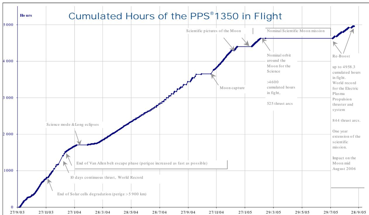
Figure 2. Total thrusting time of the Smart-1 EPS. Since the 30<sup>th</sup> of September, the EPS was used quasi-continuously. World record for Hall effect thrusters occurs in April 2004 with more than 1700 hours of operation in flight. *The longest continuous firing occurs between December 23<sup>rd</sup> and January 2<sup>nd</sup> 2004, for 240 hours(10 days)..*
