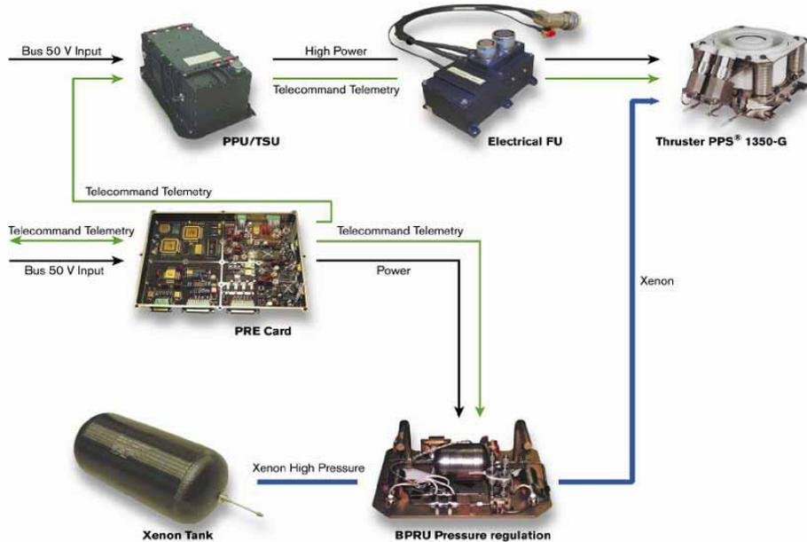
Figure 1. Sketch of the SMART-1 Electric Propulsion subSystem.
