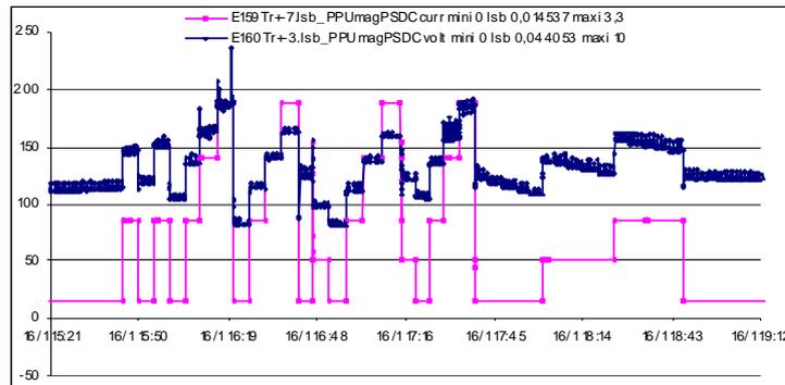
Figure 9. Magnet current during a characterisation test sequence of the EPS Smart-1 in flight.
