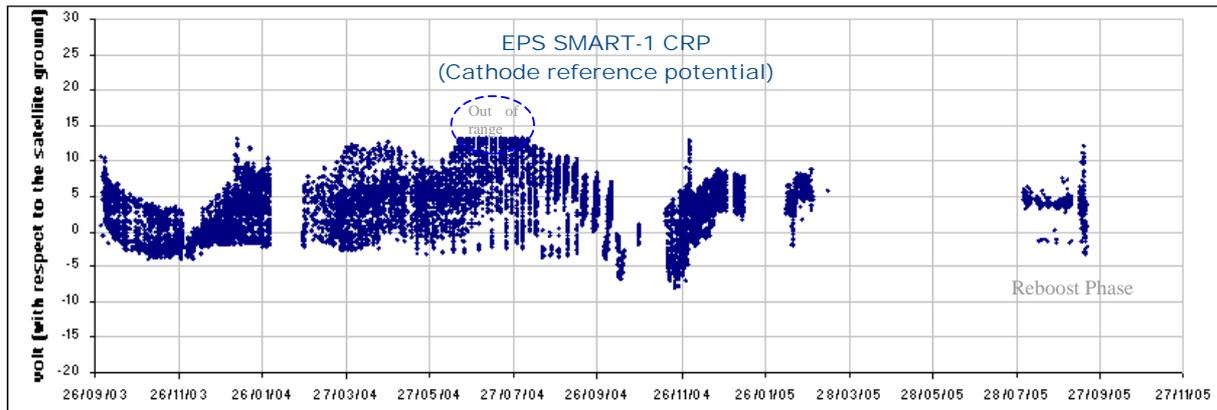
Figure 6. Long term (24 months) Cathode potential with respect to the electrical ground of the satellite.
