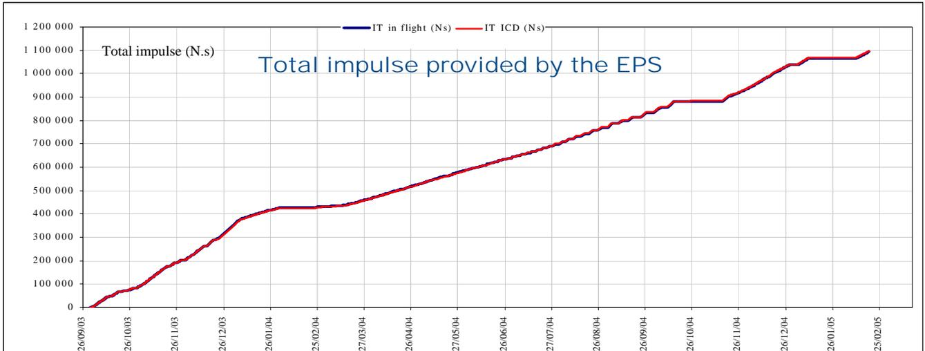
Figure 3. Total impulse comparison, measured in flight and forecasted in the Interface control document (ICD): the data are clearly superposed. EPS provided more than 1 million N.s .
