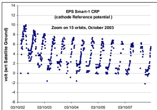
Figure 7. Zoom on 15 orbits, Cathode potential with respect to the electrical ground of the satellite.
