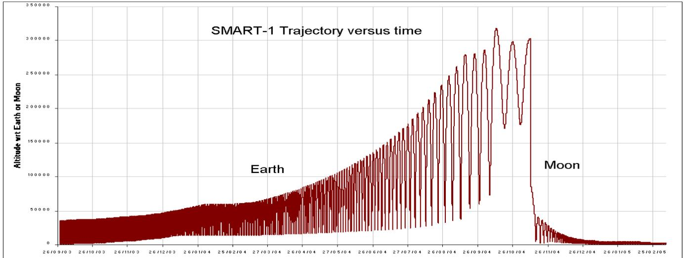
Figure 3. Orbit of the SMART-1 Satellite from Earth to the Moon. *This is the first time that a satellite follows such spiraling trajectory.*
