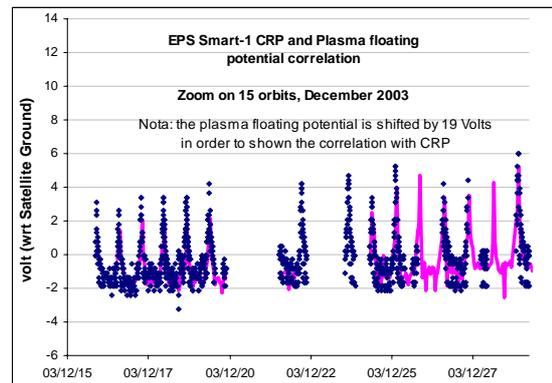
Figure 8. Correlation of the Cathode potential with the plasma potential.
