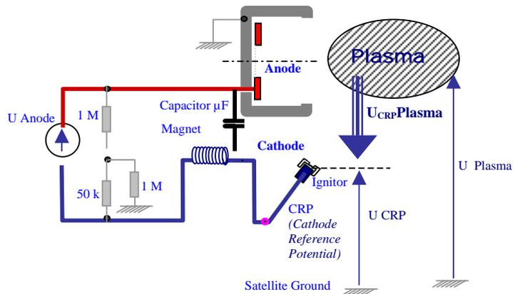
Figure 5. Sketch of the simplified electrical circuit of the EPS Smart-1. *The Cathode potential with respect to the electrical ground of the satellite is called CRP.*
