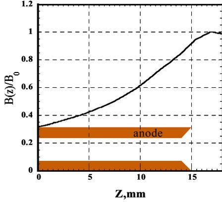
**Figure 7. Assumed magnetic flux density distribution.**
