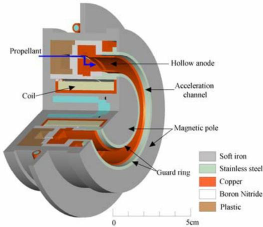
**Figure 1. The University of Tokyo Anode Layer Hall Thruster.**
