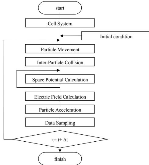
Figure 5. A flow chart of the calculation.
