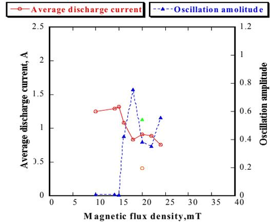
Figure 13. Computed discharge current oscillation amplitude
