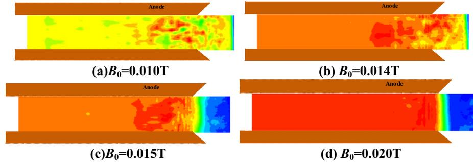
Figure 16. Computed electric potential distributions.
