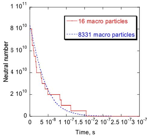
Figure 10. Neutral number history in a cell. One is a case a macro particle contains  $5.0 \times 10^9$  real neutrals. The other is  $1.0 \times 10^7$ .
