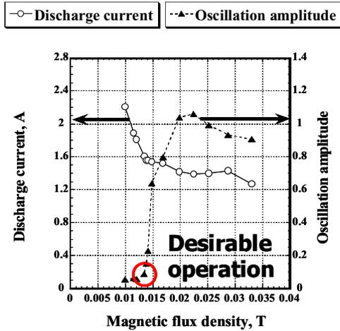
Figure 3. Oscillation characteristics.<sup>4)</sup> D=3mm, Z=1mm.
