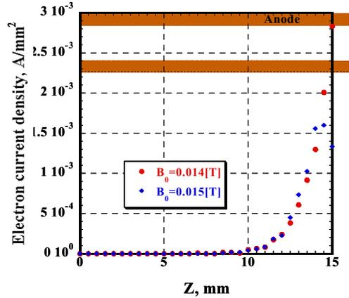
Figure 15. Discharge current distribution on the anode surface.
