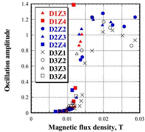
Figure 4. Relation between oscillation amplitude and B. Z=1–4mm, D=1–3mm, Vd=400V.<sup>4)</sup>
