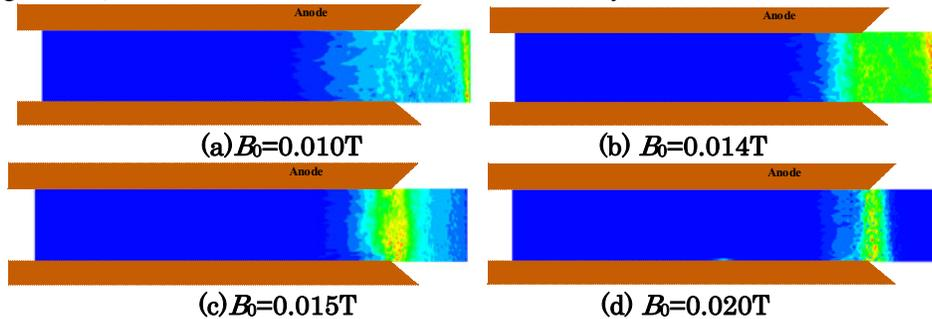
Figure 17. Computed electron temperature distributions.
