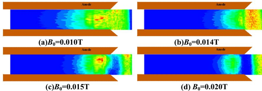
Figure 14. Computed electron number density distributions.
