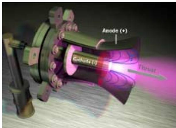
**Figure 1.** Representative schematic of the self-field magnetoplasmadynamic thruster with basic acceleration mechanism.
