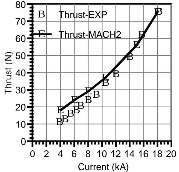
**Figure 6.** Comparisons of the MACH2- calculated thrust with experimental data for a range of discharge currents.
