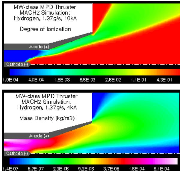
**Figure 5.** MACH2 two-dimensional distributions for the 10kA case. Top: Average degree of ionization. Bottom: Mass Density.
