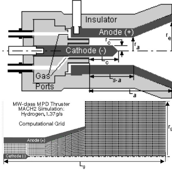
**Figure 2.** Top: Schematic of the multi-megawatt, MY-II MPD thruster used for the MACH2 simulations. Bottom: MACH2 computational region and grid. Dimensions in mm:  $r_c=4.75$ ,  $r_a=25$ ,  $r_e=52$ ,  $L_c=45$ ,  $L_{s-a}=75$ ,  $L_a=104$ ,  $L_g=300$ ,  $r_g=104$ .
