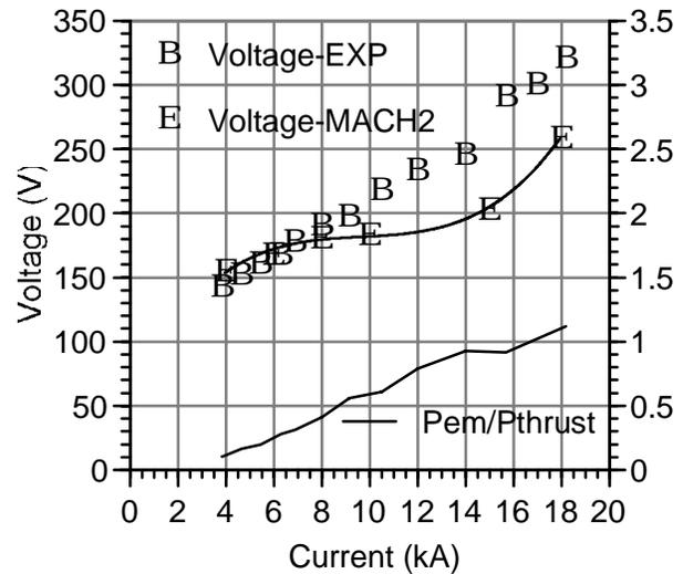
**Figure 7.** Comparisons of calculated plasma voltage to experimental total voltage. The ratio of electromagnetic thrust power to total thrust is also depicted.
