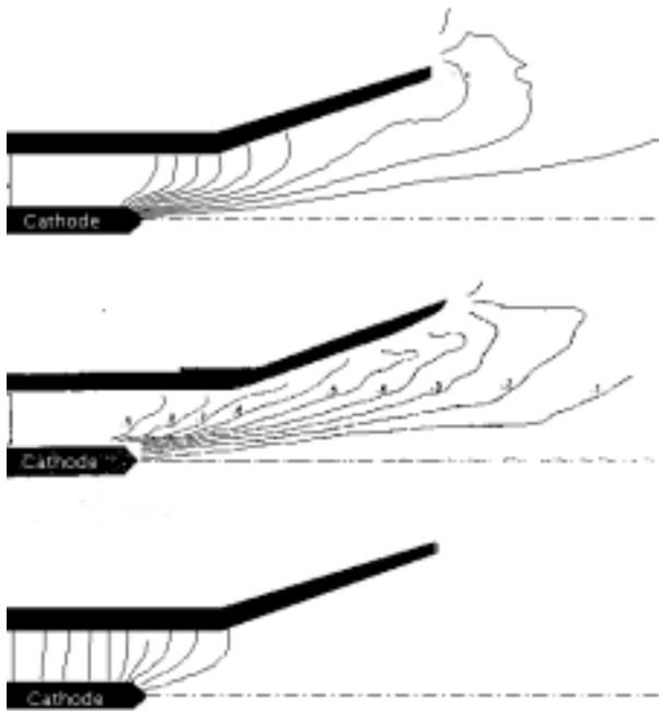
**Figure 3.** Current Distribution at 10kA. Each contour represents a 10% increment.
