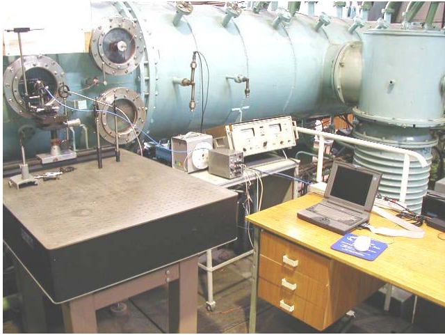
Figure 1. TSNIMASH facility #2 and diagnostic equipment during measurement of the SETAL erosion properties.
