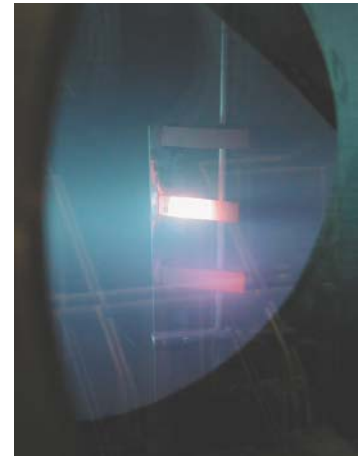
Figure 2. Samples of materials in the TAL beam.
